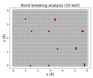
Fig. 6 MD simulation results of proton bombardment on a PTCDA molecule. Position (0, 0) represents the center of the PTCDA molecule. Each circle marks an impacting position, with red circles denoting bond breaking events.
