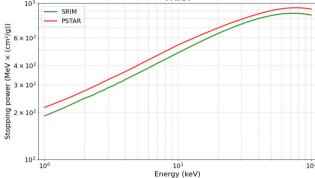
Fig. 5 Comparison of the stopping power of protons in graphite and PMMA over the kinetic energy range of 1 keV to 100 keV.
