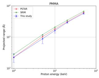
Fig. 4 Comparison of the projected range of protons in graphite and PMMA calculated in this study with reference data from PSTAR and SRIM. Error bars represent one standard deviation.
