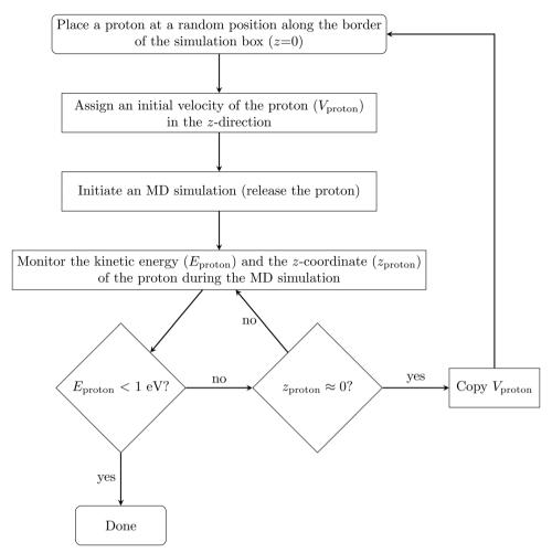
The MD workflow for simulating the projected range of a proton in a material
