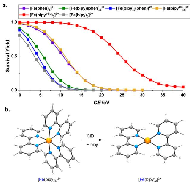
Fig. 4 (a) Breakdown curves of  $[\text{Fe}(\text{N}^{\wedge}\text{N})_3]^{2+}$  as a function of collision energy. (b) DFT-calculated structures of quintet  $[\text{Fe}(\text{bipy})_3]^{2+}$  and  $[\text{Fe}(\text{bipy})_2]^{2+}$  at the PBE/DVZP level of theory.
