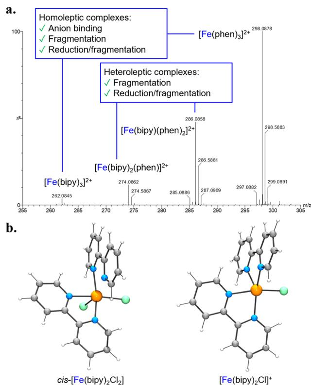
**Fig. 2** (a) Example ESI-MS of a solution containing  $[\text{Fe}(\text{bipy})_3]\text{Cl}_2$  (2  $\mu\text{M}$ ) and  $[\text{Fe}(\text{phen})_3]\text{Cl}_2$  (2  $\mu\text{M}$ ) after 4 h at 26 °C in MeOH. (b) DFT-calculated structures of high-spin *cis*- $[\text{Fe}(\text{bipy})_2\text{Cl}_2]$  and trigonal-bipyramidal  $[\text{Fe}(\text{bipy})_2\text{Cl}]^+$  at the PBE/DVZP level of theory.
