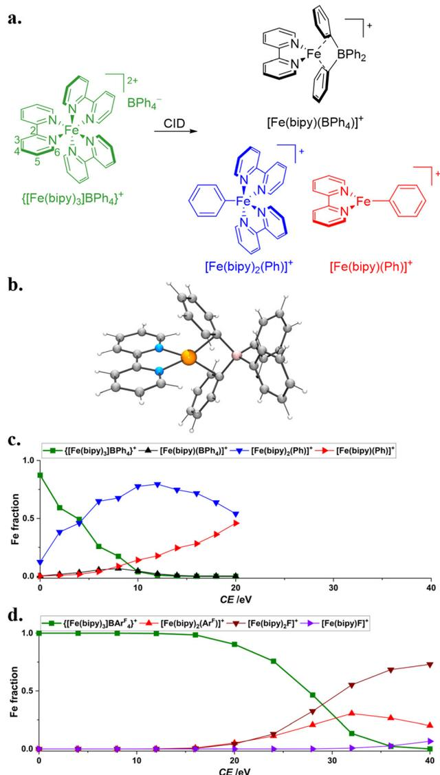
Fig. 3 (a) CID of  $\{[Fe(bipy)_3]BPh_4\}^+$  affords monocationic fragments. (b) DFT-calculated structure of high-spin  $[Fe(bipy)(BPh_4)]^+$  at the PBE/DVZP level of theory. Fe speciation during dissociation of (c)  $\{[Fe(bipy)_3]BPh_4\}^+$  and (d)  $\{[Fe(bipy)_3]BARF_4\}^+$ .
