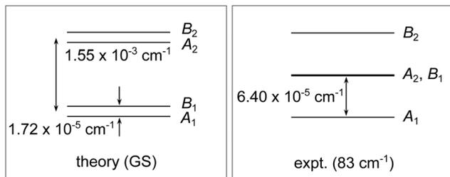
Fig. 11 A qualitative diagram of the tunneling splitting pattern of the water hexamer cage in the ground state, obtained using theory, and in the excited state at  $83\text{ cm}^{-1}$ , determined in the experiment of ref. 36.
