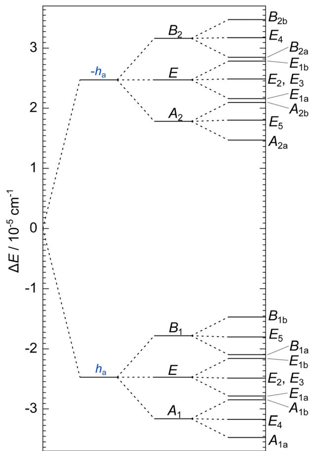
Fig. 4 Tunneling splitting pattern of the vibrational ground state of the water hexamer prism on MB-pol PES.<sup>72–74</sup> The vertical sets of levels, from the left to right, are the energy splittings due to the mechanisms: AD, AD +  $\bar{A}\bar{D}/\bar{D}A$ , and AD +  $\bar{A}\bar{D}/\bar{D}A$  + rot E + rot C, respectively. See the text for notation.
