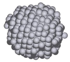
Fig. 1 Experimentally reconstructed platinum nanoparticle used in this study. The nanoparticle consists of 353 atoms and was obtained from STEM images.
