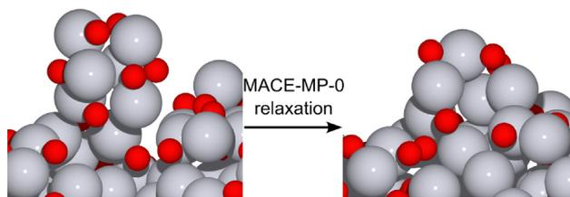
Fig. 6 Illustration of the commonly observed phenomena during a MACE-MP-0 geometry optimization, the Pt<sub>6</sub>O<sub>8</sub> species is packed back into the nanoparticle.
