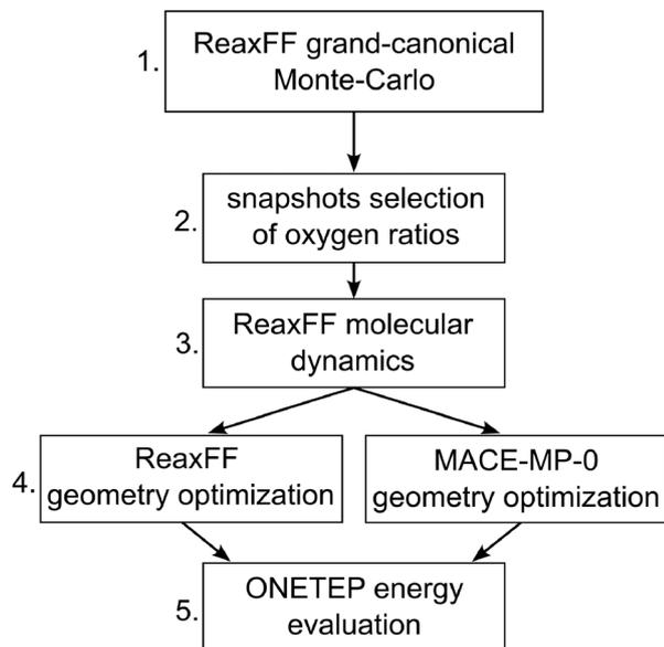
Fig. 2 The computational workflow followed in this study. Monte Carlo simulations provide initial configurations, molecular dynamics simulations are then performed to relax the geometries and further explore the phase space. Finally, ONETEP linear-scaling DFT calculations are carried out to obtain the electronic structure and refined energetics of the oxidized nanoparticles.
