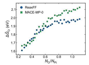
Fig. 8 Oxygen binding energy per oxygen atom plotted vs. oxygen ratio calculated using eqn (3). Two regimes can be observed, a linear, monotonic regime for ratios below 0.7, which then plateau at higher ratios. Compared to MACE-MP-0, ReaxFF predicts stronger binding at higher
