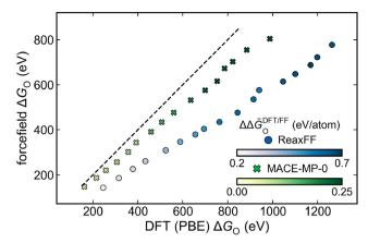
Fig. 10 Total binding energies  $\Delta G_{\rm O}$  predicted by both forcefields plotted against DFT. Colors are used to represent the binding energy difference per atom between the forcefields and DFT  $\Delta\Delta\bar{G}_{\text{O}}^{\text{DFT/FF}}.$  The dashed line serves as a reference for the perfect agreement between the forcefields and DFT.
