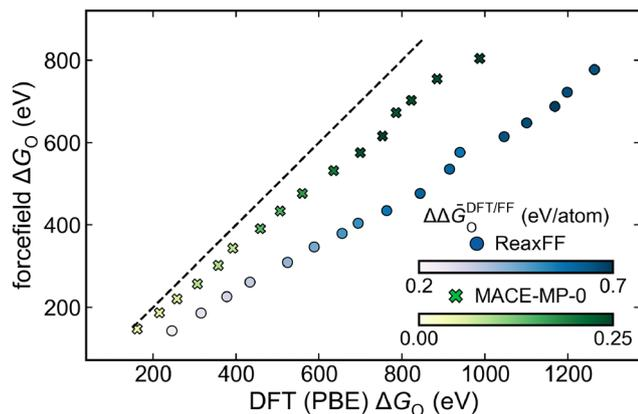
Fig. 10 Total binding energies  $\Delta G_{\text{O}}$  predicted by both forcefields plotted against DFT. Colors are used to represent the binding energy difference per atom between the forcefields and DFT  $\Delta\Delta G_{\text{O}}^{\text{DFT/FF}}$ . The dashed line serves as a reference for the perfect agreement between the forcefields and DFT.
