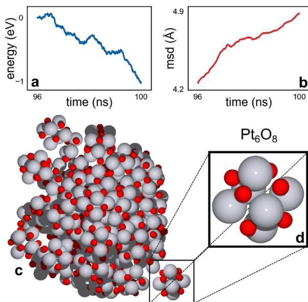
Fig. 5 An example of a dissociation event taking place during the dynamics at high oxygen fractional occupancy ( $N_{\text{O}}/N_{\text{Pt}} > 0.6$ ). These events lead to an energy reduction (a) and geometrical deformation shown by an increase in mean square deviation (msd) of nuclear coordinates (b). The final state of the nanoparticle after 100 ns is shown with an oxygen ratio of 1.07 (c). A Pt<sub>6</sub>O<sub>8</sub> species is partially detached from the nanoparticle (d).
