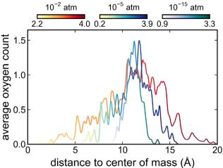
Fig. 4 Distribution of oxygen with respect to the center of mass of the oxidized nanoparticle. Subsurface and core oxygen atoms are observed as the pressure increases from  $10^{-15}$  to  $10^{-2}$  atm. No normalization has been applied. Oxygen coordination averaged over platinum atoms located around 1 Å of each radial subshell is shown as color gradient. The figure has been created by averaging over the 100 ns of NVT simulations in step 3, but is shown here for clarity
