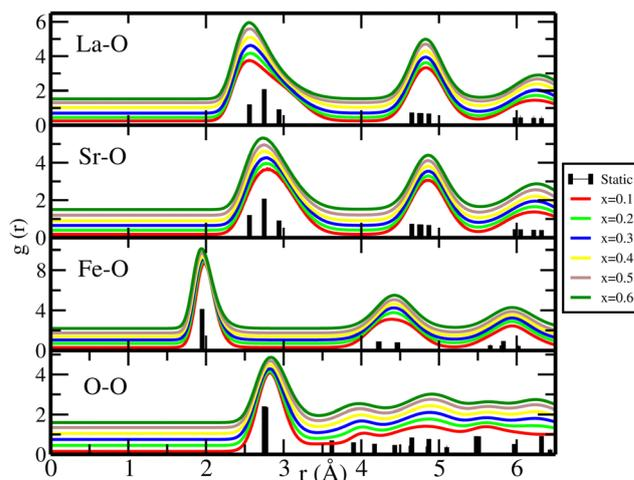
Fig. 3 The radial distribution function (RDF) between select species in  $\text{La}_{1-x}\text{Sr}_x\text{FeO}_{3-x/2}$ , where  $x = 0.1$  to  $0.6$ , from NPT-MD simulations at 1200 K. The black bars represent the corresponding X-ray locations. The plots are displaced along the y-axis for clarity.
