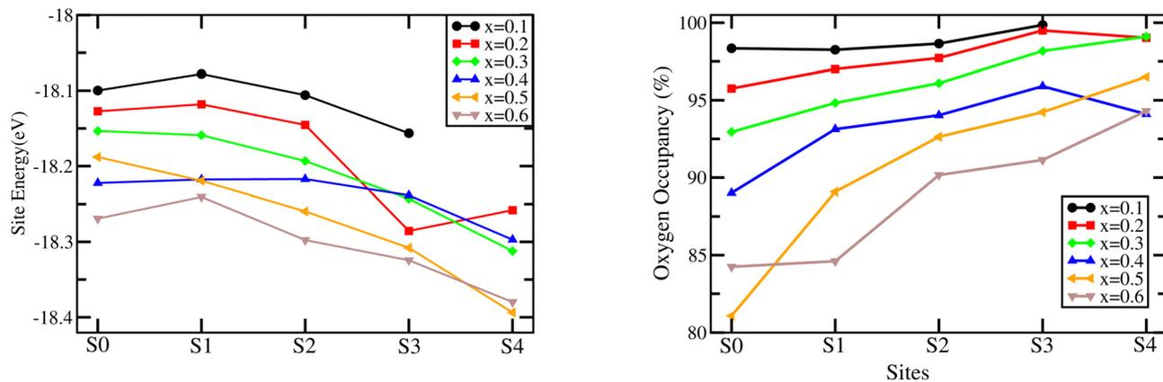
Fig. 7 Left: Site energies of oxide ions at the five different local cationic environments, S0 to S4 (where the indices mark the Sr coordination of the sites), across the composition range,  $x = 0.1$  to  $0.6$ , from NPT-MD simulations at 1200 K. Right: The corresponding oxygen occupancies in these environments.
