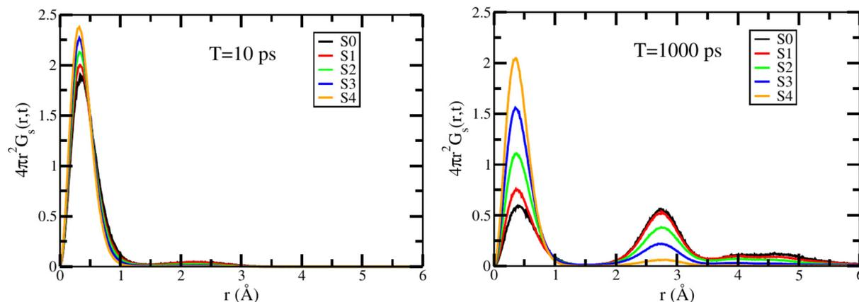
Fig. 13 The evolution of the self-part of the van-Hove correlation function of the oxide ions in  $\text{La}_{1-x}\text{Sr}_x\text{FeO}_{3-x/2}$  from the five distinct oxygen environments (S0 to S4) at two different time intervals is demonstrated for the composition  $x = 0.6$ . These profiles are averaged over the NPT-MD trajectories at 1200 K.
