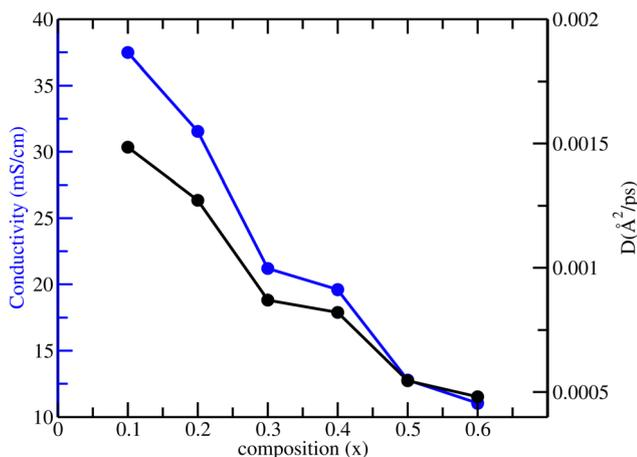
Fig. 5 The self-diffusivity of oxide ions (black) and the corresponding conductivity (blue) for  $\text{La}_{1-x}\text{Sr}_x\text{FeO}_{3-x/2}$ , where  $x = 0.1$  to  $0.6$  from NPT-MD simulations at 1200 K.
