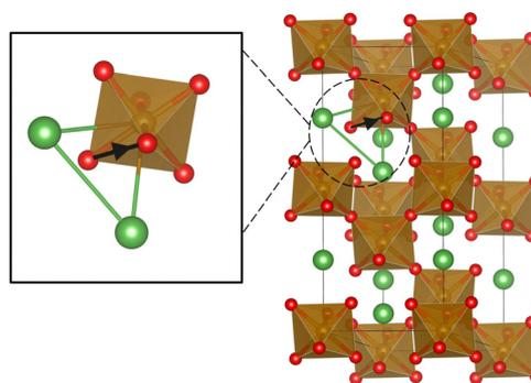
**Fig. 10** Schematic diagram of oxide ion diffusion from one site to another through a triangular bottleneck made up of two La/Sr (green) and one Fe (brown). The black arrow shows the oxygen diffusion path along the edges of the  $\text{FeO}_6$  octahedra.
