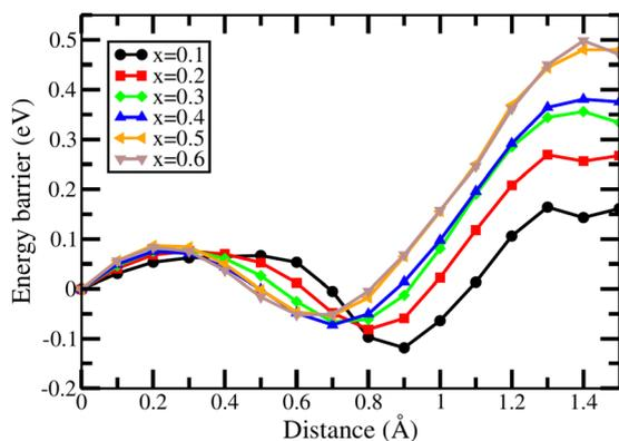
**Fig. 9** Microscopic energy profiles of oxide ion diffusion in  $\text{La}_{1-x}\text{Sr}_x\text{FeO}_{3-x/2}$ , across the compositions  $x = 0.1$  to  $0.6$ , at 1200 K. The distances are measured from the oxygen lattice site (at  $x = 0$ ) and shown up to the transition state (saddle point), at  $x = 1.5$ .
