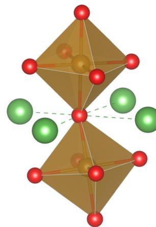
Fig. 6 The local cationic environment around the oxygens (red), shared by two  $\text{FeO}_6$  octahedra (Fe is located at the center of the octahedra). The locally four coordinated cations ( $\text{La}^{3+}/\text{Sr}^{2+}$ ) are shown as green balls.
