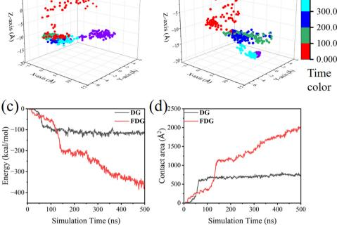
Fig. 4 Centroid migration path of the RBD on the (a) DG and (b) FDG during 500 ns. The corresponding Z-axis coordinates of investigated materials is approximately -36.5 Å. (c) Interaction energy and (d) contact area between the RBD and the investigated materials
