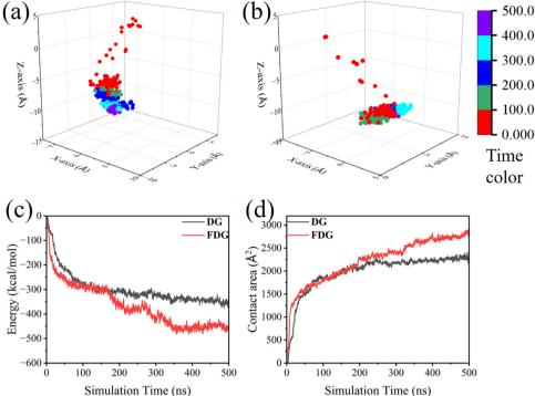
Fig. 5 Centroid migration path of M<sup>pro</sup> on the (a) DG and (b) FDG over 500 ns. The corresponding Z-axis coordinates of the investigated materials is approximately -25.2 Å. (c) Interaction energy and (d) contact area between M<sup>pro</sup> and the investigated materials.
