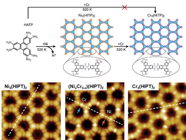
Fig. 14 Structural transformation by metal substitution from  $Ni_3(HITP)_2$  through  $(Ni_xCr_{3-x})(HITP)_2$ , eventually to  $Cr_3(HITP)_2$  frameworks on Au(111) in response to the addition of Cr atoms. Reproduced with permission.<sup>170</sup> Copyright 2023 Wiley-VCH GmbH.
