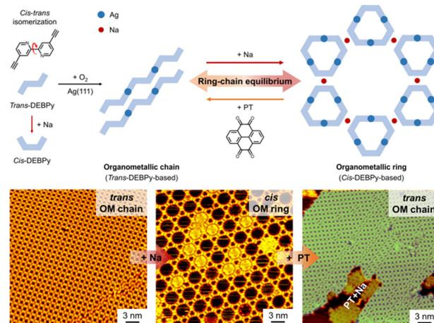
Fig. 8 Ring-chain equilibrium between covalent organometallic chains and rings induced by the regulation of weak intermolecular interactions provided by Na. Reproduced with permission.<sup>132</sup> Copyright 2024 American Chemical Society.
