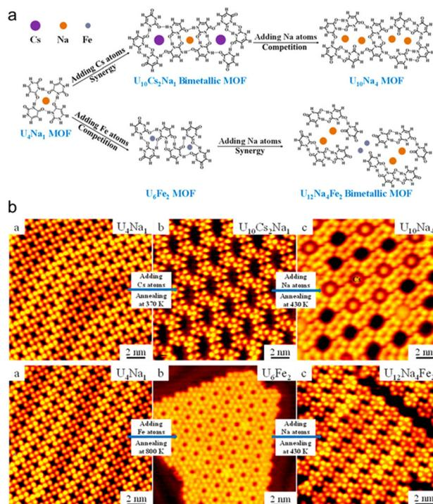
Fig. 13 Structural transformation of different 2D metal-organic networks on Au(111), including two bimetallic structures. (a) Illustration of the formation of  $U_4Na_1$ ,  $U_{10}Cs_2Na_1$ ,  $U_{10}Na_4$ ,  $U_6Fe_2$ , and  $U_{12}Na_4Fe_2$  structures. (b) Structural transformations starting from the  $U_4Na_1$  structure induced by Cs and Fe, respectively. Reproduced with permission.<sup>43</sup> Copyright 2021 American Chemical Society.
