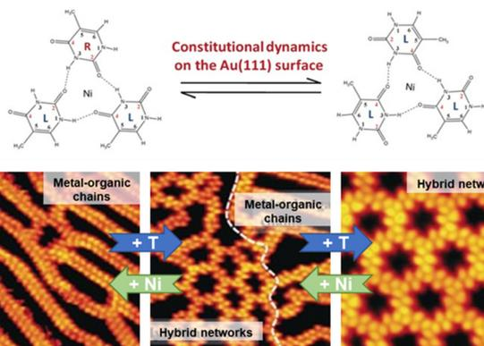
Fig. 9 Reversible structural transformation of Ni-based metal-organic nanostructures on Au(111) in response to additional T molecules or Ni atoms. Reproduced with permission.<sup>139</sup> Copyright 2016 WILEY-VCH Verlag GmbH & Co. KGaA, Weinheim.
