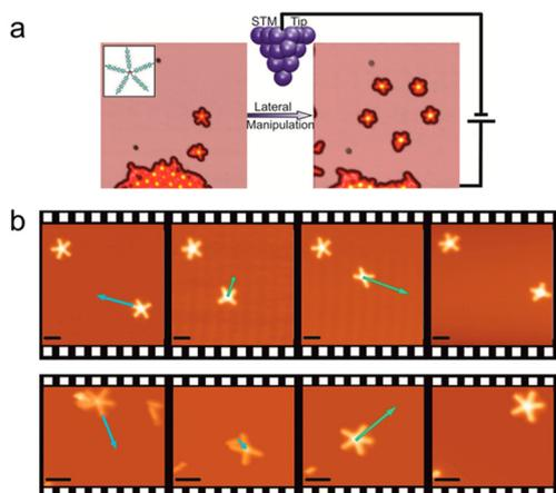
Fig. 12 Structural transformation of Gd-supramolecules induced by STM lateral manipulations on Ag(111). (a) Formation of a pentagon by displacing five pentamers. (b) *In situ* tailoring and displacement of Gd-carbonitrile metal-organic supramolecules. Reproduced with permission.<sup>154</sup> Copyright 2014 American Chemical Society.
