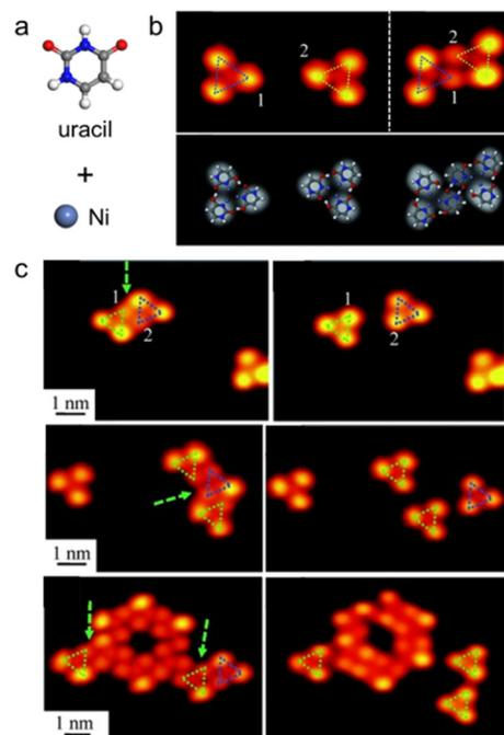
Fig. 10 Structural transformation of metal-organic clusters on Au(111) induced by STM manipulation. Reproduced with permission.<sup>144</sup> Copyright 2015 Wiley-VCH Verlag GmbH & Co. KGaA, Weinheim.
