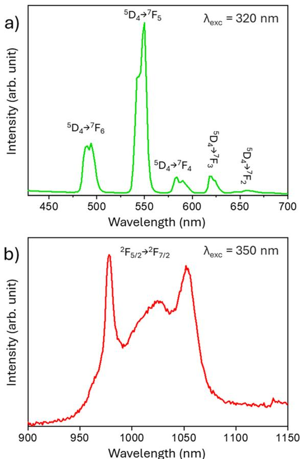
Fig. 6 Emission spectra of **2** (a) and **1** (b) at the indicated  $\lambda_{\text{exc}}$  in solid state at room temperature.
