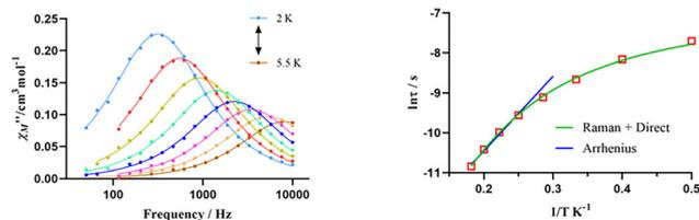
Fig. 4 (left) Frequency dependence of the  $\chi_M''$  signals at different temperatures for **1** under a field of 0.1 T. The solid lines represent the best fitting to the Debye model. (right) Representation of  $\ln\tau$  vs.  $1/T$  for **1** at 0.1 T. The solid lines represent the best fit of the experimental data to the Arrhenius equation for a thermally activated process (blue) or for a combination of Raman and Direct relaxation processes (green).
