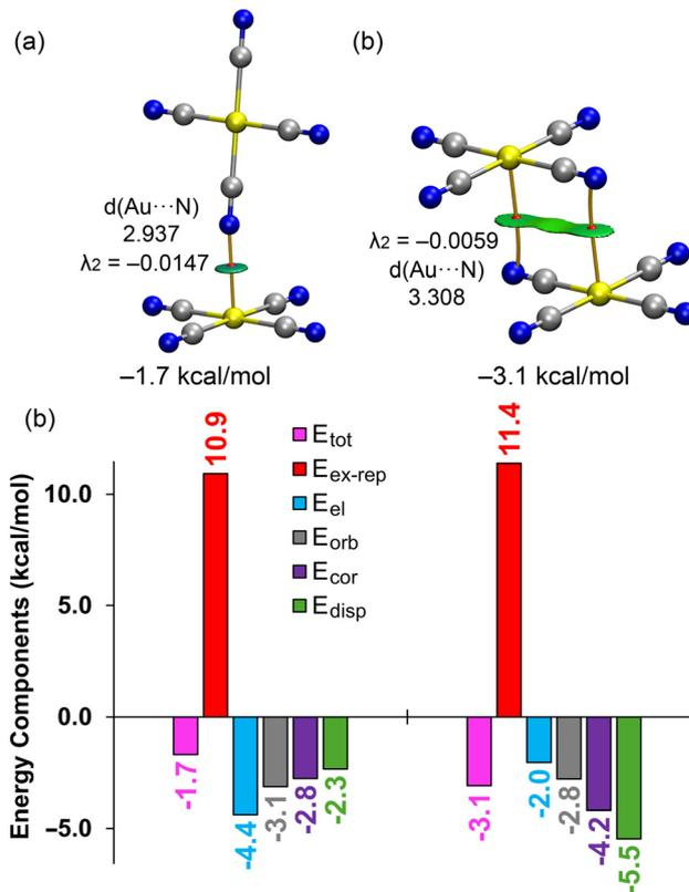
Fig. 11 Top: QTAIM/NCIplot analysis of the T-shape (a) and antiparallel (b) anion...anion dimers of  $[\text{Au}(\text{CN})_4]^-$ . Bottom: EDA analysis of both dimers, total energy ( $E_{\text{tot}}$ ) in pink, electrostatic ( $E_{\text{el}}$ ) in blue, exchange repulsion ( $E_{\text{ex-rep}}$ ) in red, orbital ( $E_{\text{orb}}$ ) in grey, correlation ( $E_{\text{cor}}$ ) in purple and dispersion ( $E_{\text{disp}}$ ) in green.
