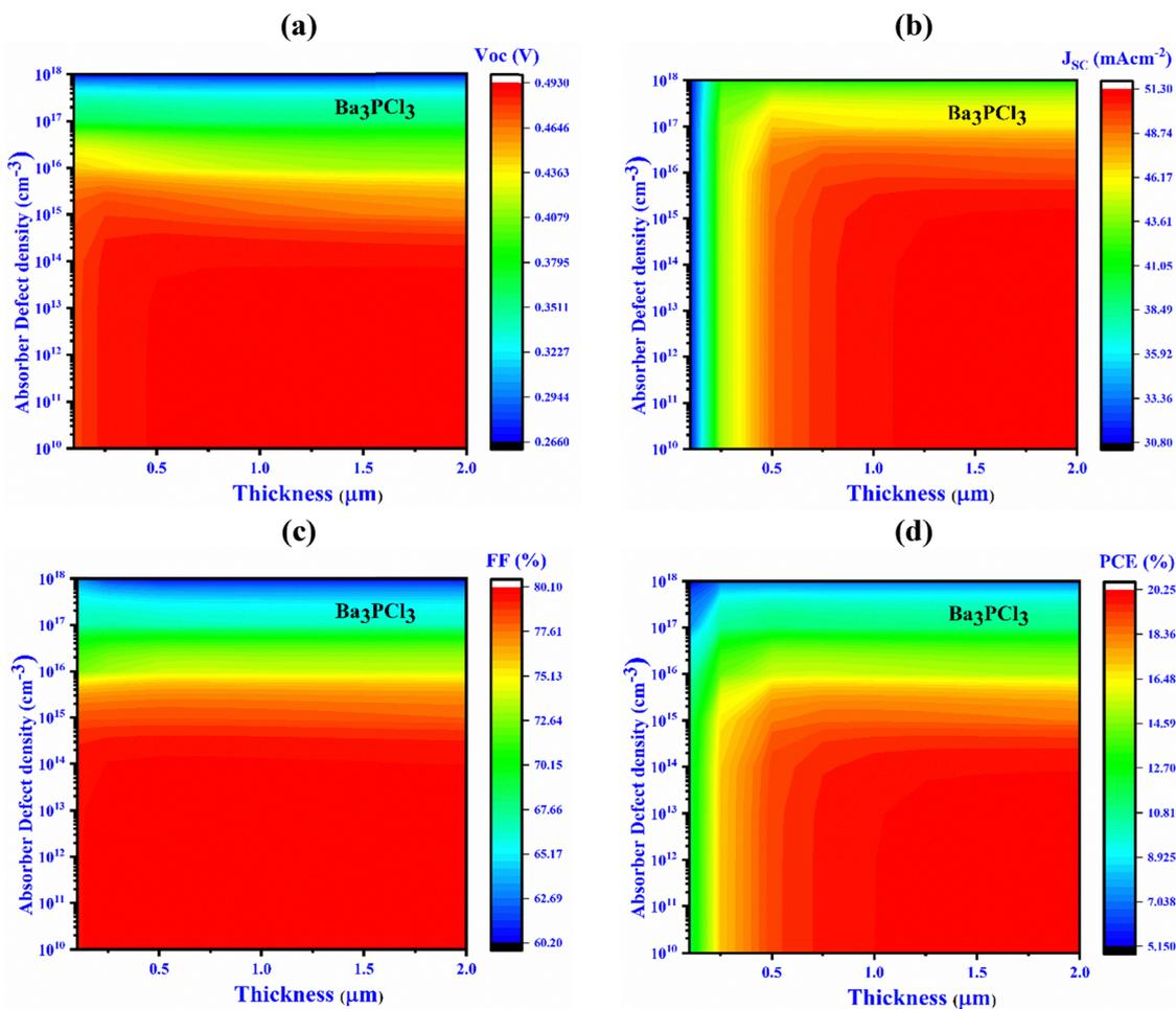
Fig. 6 Influence of variations in absorber thickness and defect density (device II,  $\text{Ba}_3\text{PbCl}_3$ ) on key PV performance factors: (a)  $V_{\text{OC}}$ , (b)  $J_{\text{SC}}$ , (c) FF, and (d) PCE.
