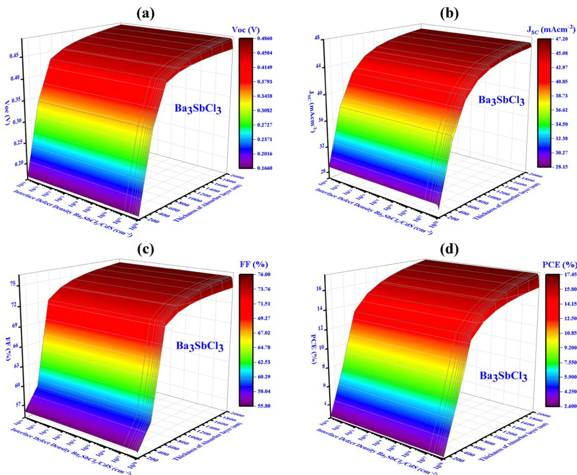
Fig. 12 Influence of variations in absorber thickness and defect interface density (device-IV, Ba<sub>3</sub>SbCl<sub>3</sub>) on key PV performance factors: (a)  $V_{OC}$ , (b)  $J_{SC}$ , (c) FF, and (d) PCE.
