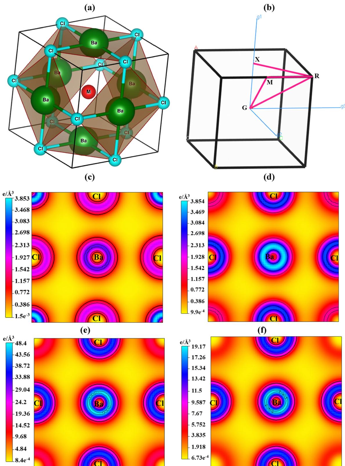
Fig. 1 (a) Crystal structure of  $\text{Ba}_3\text{MCl}_3$  ( $\text{M} = \text{N}, \text{P}, \text{As}, \text{and Sb}$ ), (b) BZ path ( $\text{X-R-M-G-R}$ ) and the distribution of electronic charges in (c)  $\text{Ba}_3\text{NCl}_3$ , (d)  $\text{Ba}_3\text{PCl}_3$ , (e)  $\text{Ba}_3\text{AsCl}_3$  and (f)  $\text{Ba}_3\text{SbCl}_3$ .
