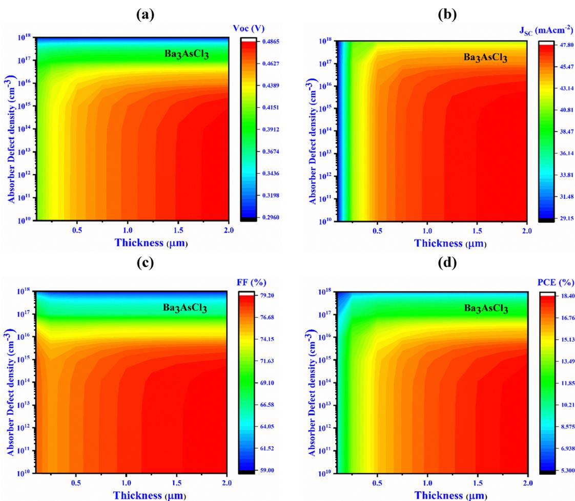
Fig. 7 Influence of variations in absorber thickness and defect density (device-III,  $\text{Ba}_3\text{AsCl}_3$ ) on key PV performance parameters: (a)  $V_{\text{OC}}$ , (b)  $J_{\text{SC}}$ , (c) FF, and (d) PCE.
