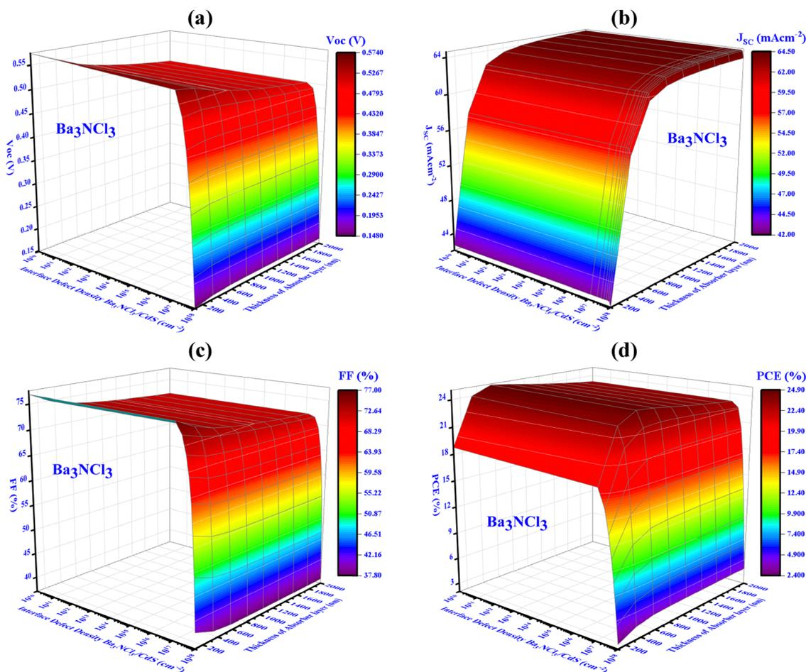
Fig. 9 Influence of variations in absorber thickness and defect interface density (device-I,  $\text{Ba}_3\text{NCl}_3$ ) on key PV performance factors: (a)  $V_{OC}$ , (b)  $J_{SC}$ , (c) FF, and (d) PCE.
