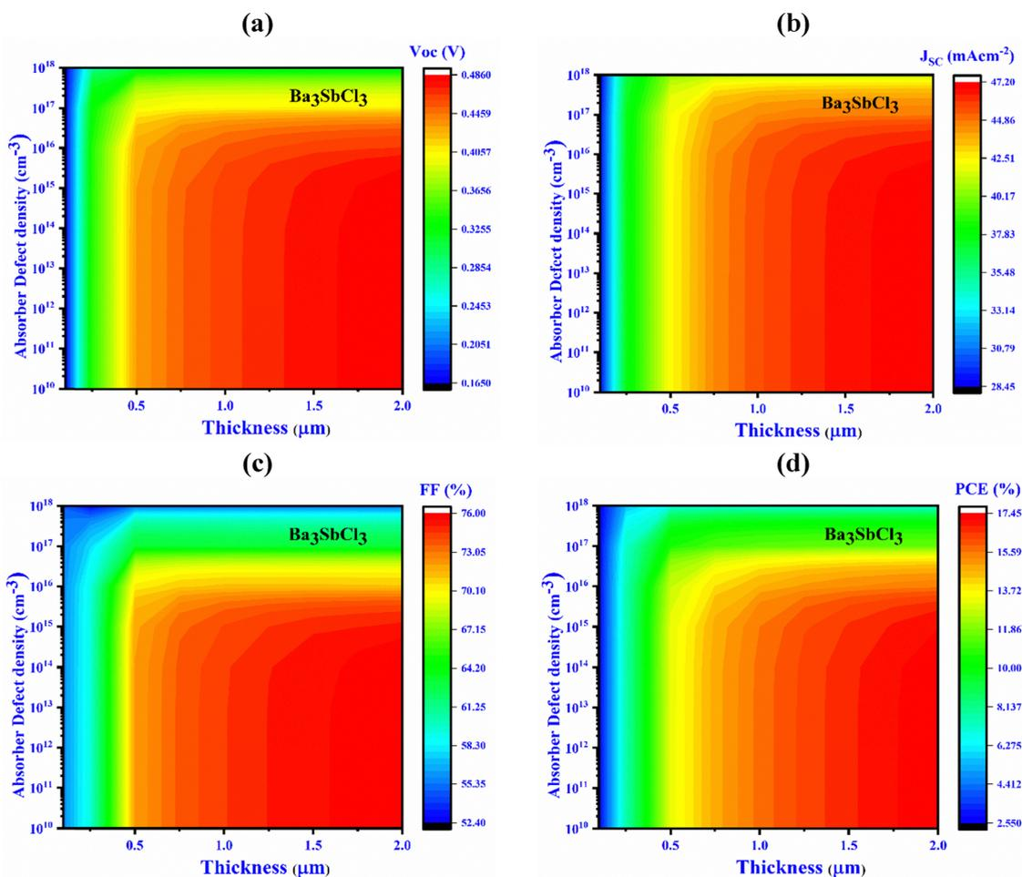
Fig. 8 Influence of variations in absorber thickness and defect density (device-IV, Ba<sub>3</sub>SbCl<sub>3</sub>) on key PV performance parameters: (a)  $V_{OC}$ , (b)  $J_{SC}$ , (c) FF, and (d) PCE.
