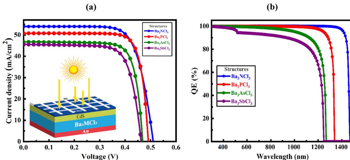
Fig. 13 (a)  $J$ - $V$  and (b) PSC QE curves for devices I, II, III, and IV.
