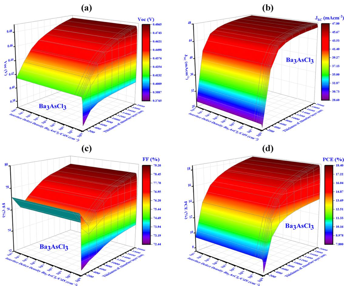
Fig. 11 Influence of variations in absorber thickness and defect interface density (device-III,  $\text{Ba}_3\text{AsCl}_3$ ) on key PV performance factors: (a)  $V_{\text{OC}}$ , (b)  $J_{\text{SC}}$ , (c) FF, and (d) PCE.
