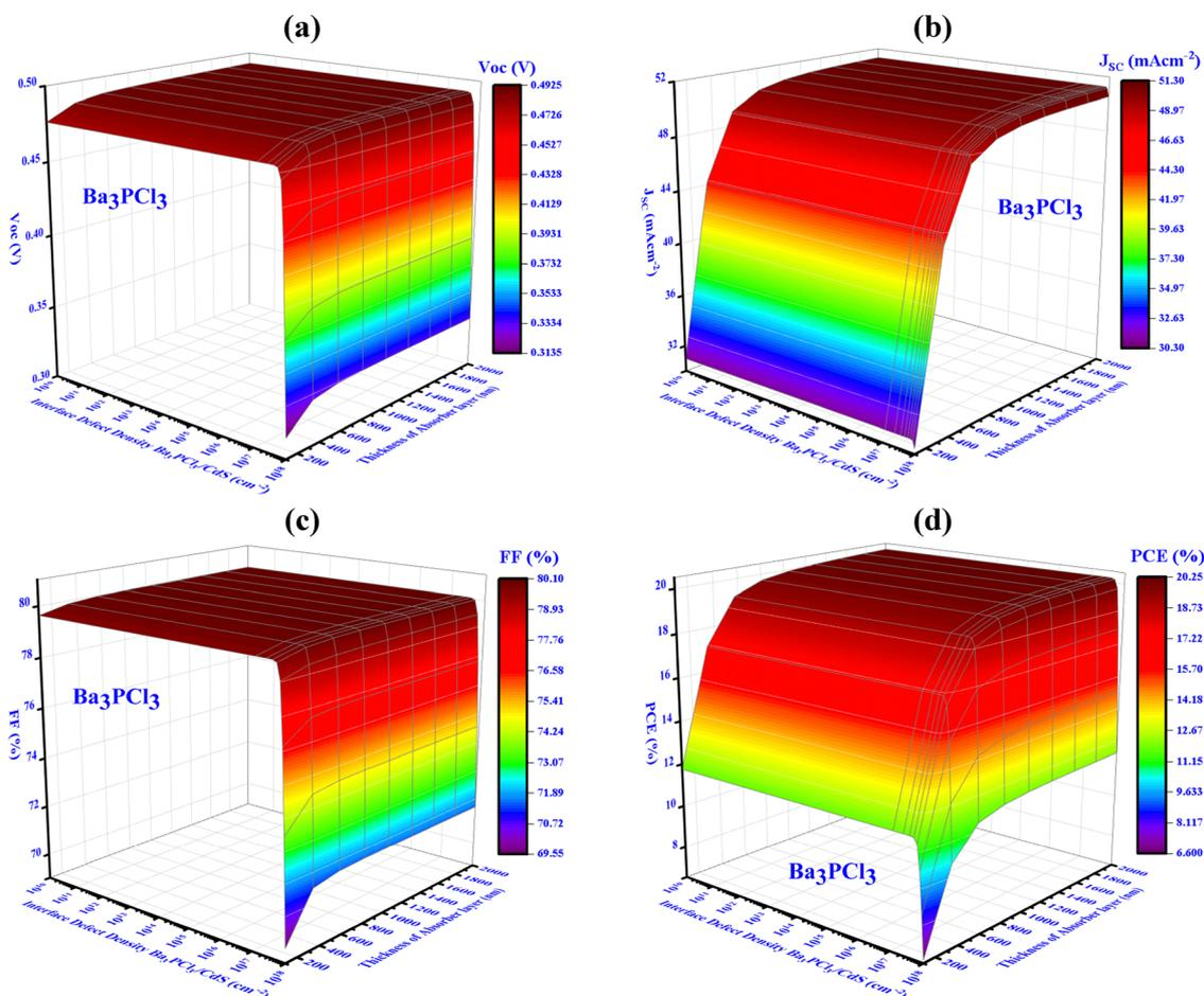
Fig. 10 Influence of variations in absorber thickness and defect interface density (device-II,  $\text{Ba}_3\text{PbCl}_3$ ) on key PV performance factors: (a)  $V_{\text{OC}}$ , (b)  $J_{\text{SC}}$ , (c) FF, and (d) PCE.
