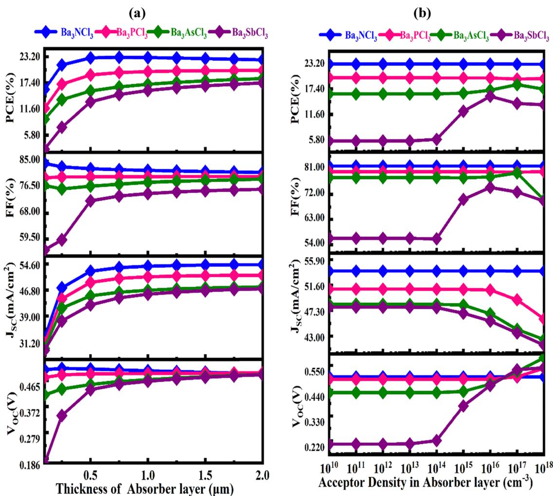
Fig. 4 Influence of alteration of the absorber layer (Ba<sub>3</sub>NCl<sub>3</sub>, Ba<sub>3</sub>PbCl<sub>3</sub>, Ba<sub>3</sub>AsCl<sub>3</sub> and Ba<sub>3</sub>SbCl<sub>3</sub>) (a) thickness and (b) acceptor density with PV factors of  $V_{oc}$ ,  $J_{sc}$ , FF and PCE.
