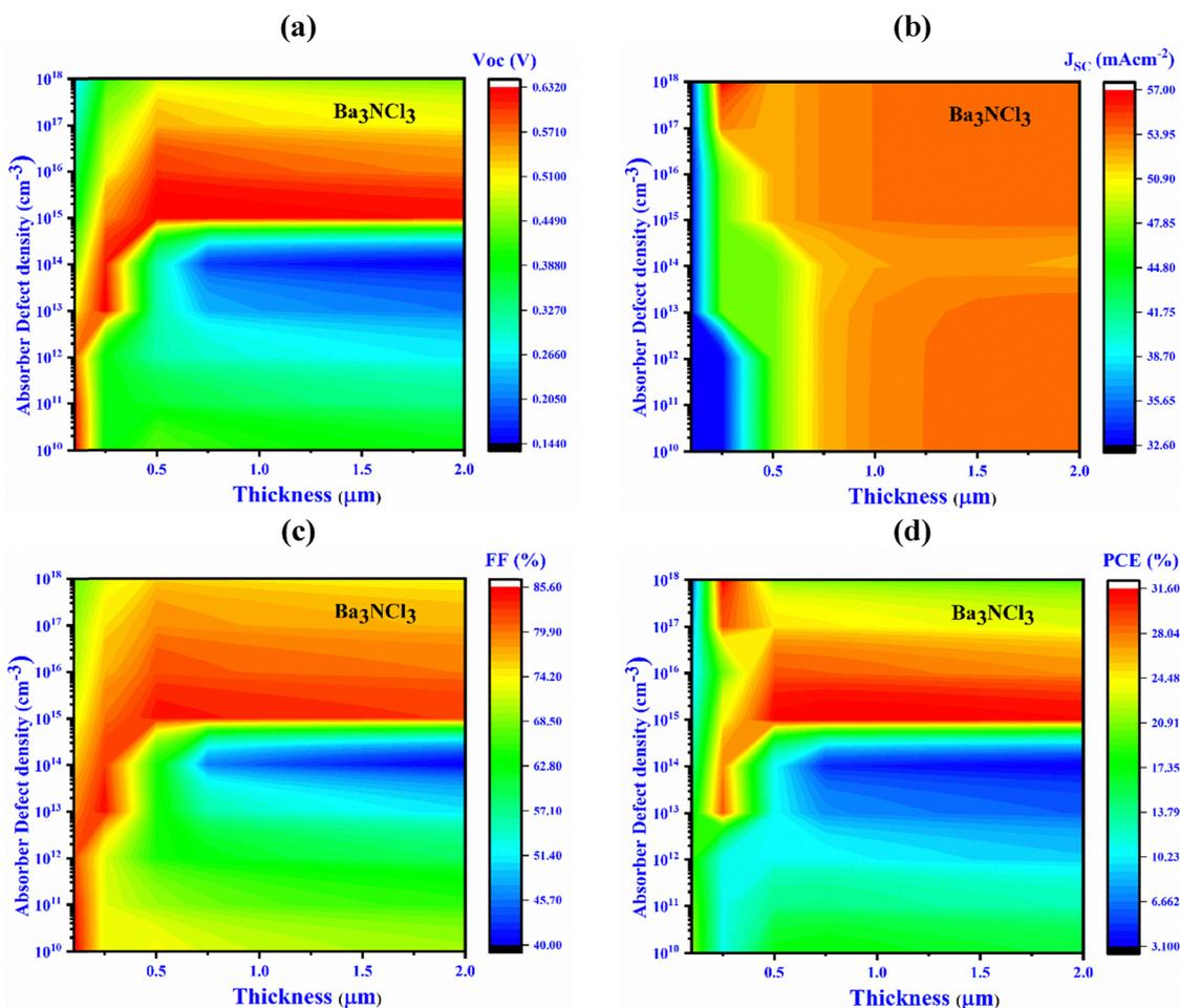
**Fig. 5** Influence of variations in absorber thickness and defect density (device-I,  $\text{Ba}_3\text{NCl}_3$ ) on key PV performance factors: (a)  $V_{\text{oc}}$ , (b)  $J_{\text{sc}}$ , (c) FF, and (d) PCE.
