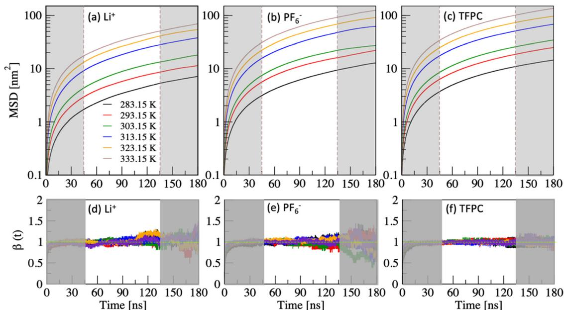
Fig. 7 Semi-log plot of MSDs (a)–(c) and corresponding values of  $\beta$  (d)–(f). The unshaded parts, the diffusive regions of the trajectories, were used to calculate the transport properties of the electrolytes.
