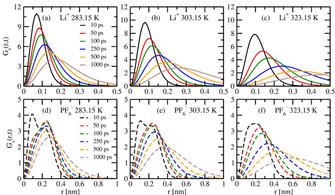
Fig. 8 Panels (a), (b) and (c) show the van Hove function of Li<sup>+</sup> at 283.15, 303.15, and 323.15 K, respectively; (d), (e) and (f) show the van Hove function of PF<sub>6</sub><sup>-</sup> at 283.15, 303.15 and 323.15 K, respectively, for six different time intervals.
