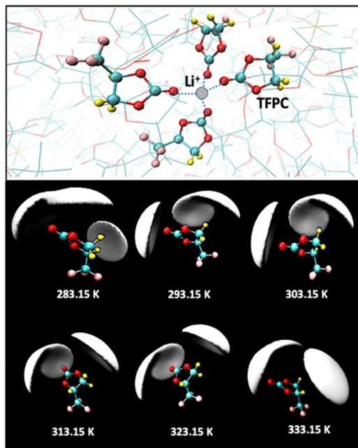
Fig. 4 A particular configuration of Li-ion interactions with TFPC is shown in the upper panel. The spatial distribution functions of Li<sup>+</sup> around TFPC at various temperatures are shown in the lower panel. The isosurface density value is 1.5 pm<sup>-3</sup>.
