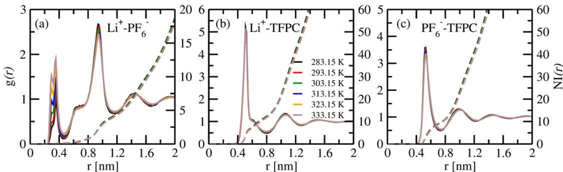
Fig. 2 The centre of mass radial distribution functions of (a)  $\text{Li}^+$ - $\text{PF}_6^-$ , (b)  $\text{Li}^+$ -TFPC, and (c)  $\text{PF}_6^-$ -TFPC pairs, and the dashed line shows the number integrals of the same at six different temperatures.
