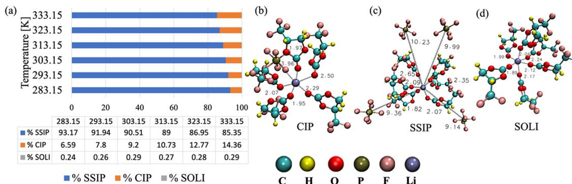
Fig. 5 (a) Percentage of Li<sup>+</sup> forming different microstructures present in the bulk electrolyte at various temperatures, (b) example of contact ion pair (CIP), (c) solvent separated ion pair (SSIP), and (d) example of solvated Li<sup>+</sup> (SOLI).
