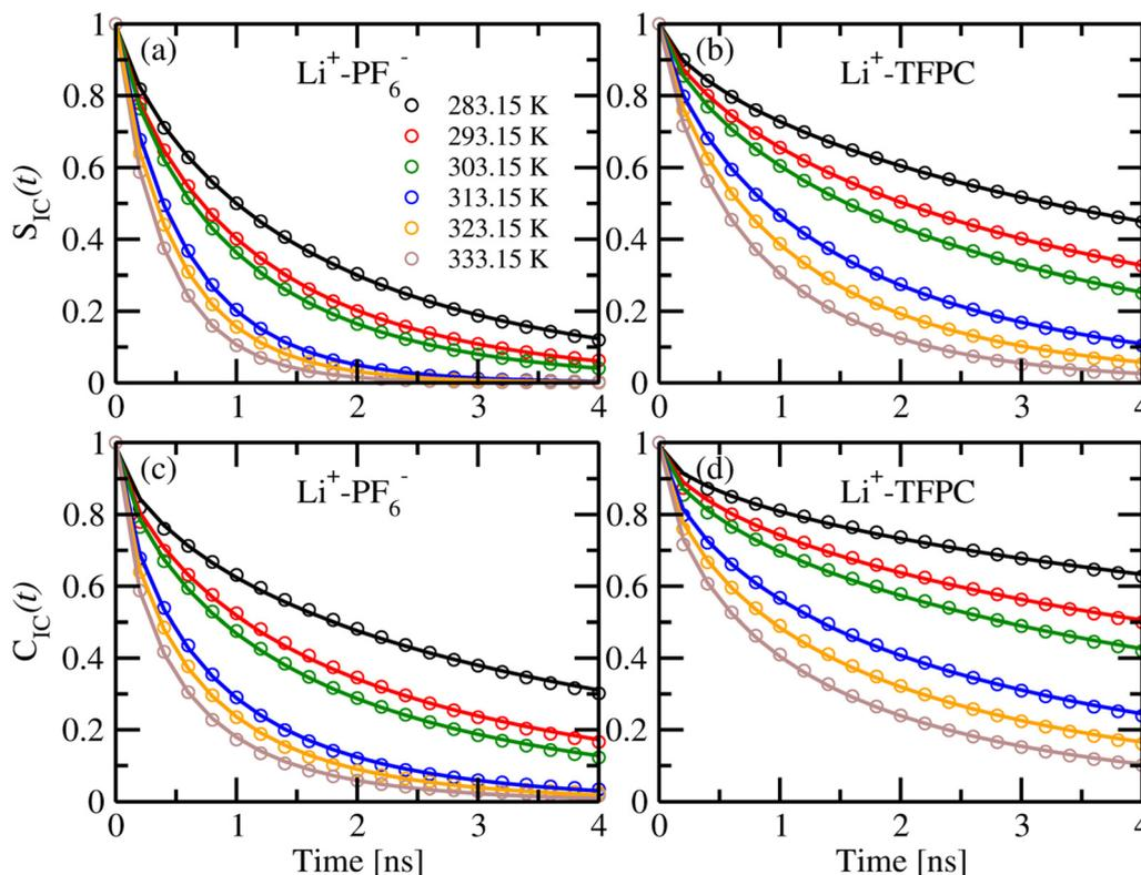
Fig. 12 Continuous ion-cage auto correlation functions of (a)  $\text{Li}^+$ -COM( $\text{PF}_6^-$ ) and (b)  $\text{Li}^+$ -COM(TFPC); intermittent ion-cage autocorrelation functions (c)  $\text{Li}^+$ -COM( $\text{PF}_6^-$ ) and (d)  $\text{Li}^+$ -COM(TFPC) at six different temperatures. The solid lines show the fitting data.
