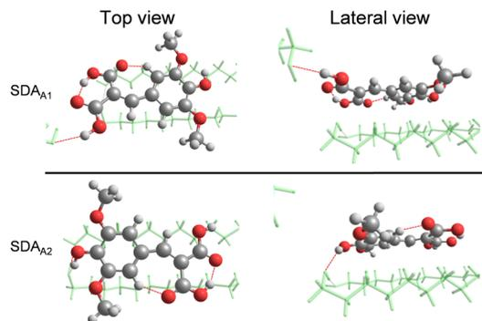
Fig. 4 Optimized ground state geometries of SDA<sub>A</sub> deposited on the model surface. Red lines denote the hydrogen bonds. The subscripts A1 and A2 refer to different binding arrangements of SDA on the model surface.
