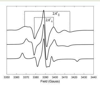
Fig. 6 Top line: EPR spectrum predicted from MD trajectory of 5-PC probes in POPC bilayer-doped with 1% mol of (LA)<sub>12</sub> and at T = 330 K. Middle and bottom lines correspond to EPR spectra predicted from BD trajectories generated from the model of rotational diffusion in the axially symmetric potential with  $\tau_c$  = 1 ns and  $\bar{C}$  = 1 and  $\tau_c$  = 0.2 ns and  $\bar{C}$  = 3, respectively (see the text for details).
