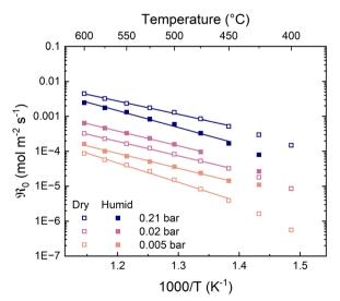
Fig. 10 Comparison of the oxygen exchange rate of BGLC37 in dry and humid carrier gases (0.03 bar H<sub>2</sub>O). The solid lines are linear fits
