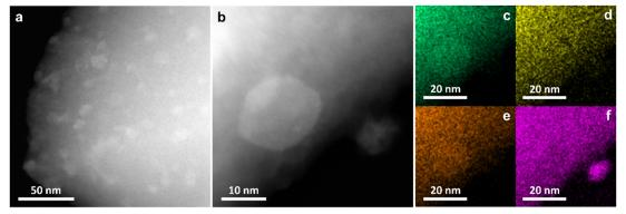
Fig. 2 (a) and (b) high-angle annular dark field (HAADF) micrographs of the BGLC37 sample showing nanoparticles distributed over the surface. (c)-(f) Elemental maps of Ba (green), Gd (yellow), La (orange), and Co (pink), respectively, derived from micrograph (b), illustrating elemental distribution.
