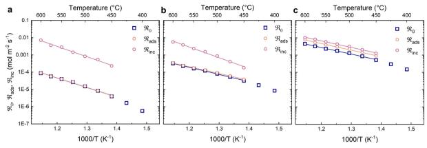
Fig. 4 Oxygen exchange rate  $(\Re_0)$  and the contributions from dissociative adsorption  $(\Re_{ads})$  and incorporation  $(\Re_{inc})$  at different oxygen partial pressures (dry carrier gas); (a) 0.005 bar (b) 0.02 bar (c) 0.21 bar. The solid lines are linear fits.
