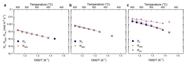
Fig. 7 Oxygen exchange rate  $(\Re_0)$  and the contributions from dissociative adsorption  $(\Re_{ads})$  and incorporation  $(\Re_{inc})$  at different oxygen partial pressures with humid carrier gas (0.03 bar  $H_2O$ ): (a) 0.005 bar (b) 0.02 bar (c) 0.21 bar. The solid lines are linear fits
