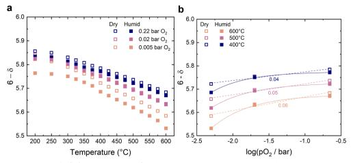
Fig. 9 Oxygen non-stoichiometry of BGLC37 measured by TG with the same temperature program as for the PIE measurements as a function of (a) temperature and (b)  $pO_2$  in dry (open symbols) and humidified (0.03 bar  $H_2O$ ) atmospheres (filled symbols). The solid and dashed lines are guides to the eve
