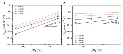
Fig. 6 Oxygen partial pressure dependencies in dry carrier gas of (a) the dissociative adsorption rate, and (b) the incorporation rate. The solid lines are linear fits.
