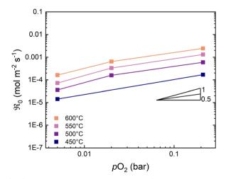
Fig. 8 Oxygen exchange rate as a function of  $pO_2$  with humid carrier gas (0.03 bar H<sub>2</sub>O).
