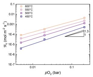
Fig. 5 Oxygen exchange rate as a function of  $pO_2$  at 400–600 °C in dry carrier gas. The solid lines are linear fits.
