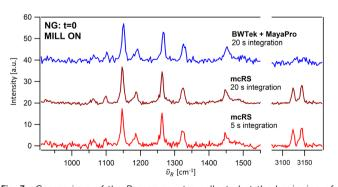
Fig. 3 Comparison of the Raman spectra collected at the beginning of milling of imidazole with the standard fiber-optics Raman system using 20 s integration (blue), and with mcRS using 20 s integration (dark red) and 5 s integration (red). Power of the excitation source: 300 mW for fiberoptics spectrometer and 25 mW for mcRS.
