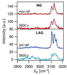
Fig. 6 Raman spectra in high-frequency region of the **moc** product (dark red and red line) and of the zni product (dark blue and light blue line): taken ex situ with a commercial research grade Raman system (moc ref and zni ref) and in situ with our mechanochemical Raman system at the end of the NG and the LAG reactions (3600 s red and light blue, respectively).
