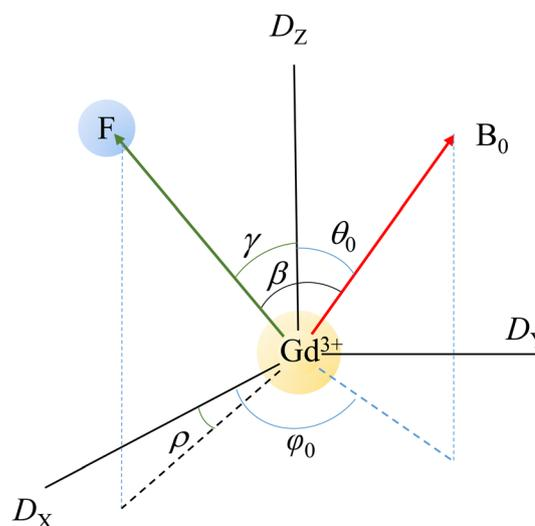
**Scheme 1** Definitions of angles used in this work.  $D_X$ ,  $D_Y$  and  $D_Z$  are the principal axes of the (molecular) ZFS frame,  $B_0$  is the direction of the spectrometer's magnetic field, and the green arrow is the direction of Gd-F vector in the molecular frame.
