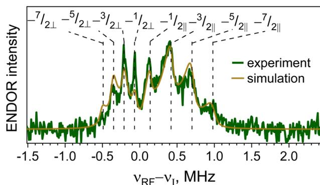
**Fig. 4** The  $^{19}\text{F}$ -ENDOR spectrum of 3-FBA/Gd- $\beta$ -CD, recorded 8 K and at field position d (see Fig. 3B). Singularities corresponding to parallel and perpendicular orientations of the corresponding  $m_s \rightarrow m_s + 1$  transitions are shown with dashed lines. Simulation with parameters given in Table 2 are shown in brown.
