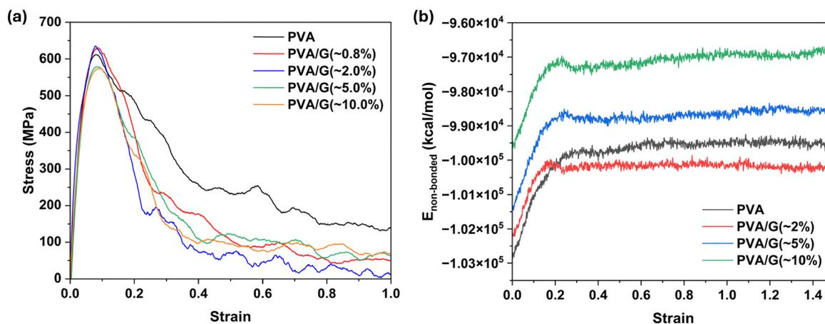
Fig. 3 (a) Comparison of stress–strain responses of the PVA and the graphene-reinforced PVA nanocomposites due to the uniaxial tension with a strain rate of  $1.5 \times 10^8 \text{ s}^{-1}$  along the Cartesian  $X$ -axis of the simulation cell. (b) Illustration of changes in non-bonded energy ( $E_{\text{non-bonded}}$ ) as a function of strain for the PVA and the G-PVA nanocomposite comprising 2–10% graphene nanofiller.
