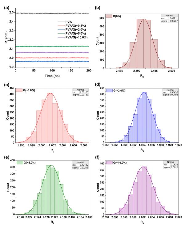
Fig. 2 Representation of the (a) temporal evolution of radii of gyration ( $R_{\rm q}$ ) and (b)–(f) normal distribution of computed  $R_{\rm q}$  values overlaid on a histogram or binned data [the inset shows values of "mu" indicating the average or expected value of the distribution and "sigma" reflecting the standard deviation], as a function of the proportion of graphene nanofiller present in the G-PVA composites, as acquired from the 200 ns of the production MD trajectory at 300 K.
