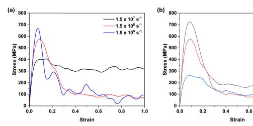
Fig. 5 Illustration of computed stress-strain curves for the 10% graphene-filled PVA nanocomposite (a) obtained by uniaxial tension at 300 K with three different strain rates viz.  $1.5 \times 10^7$  s<sup>-1</sup>,  $1.5 \times 10^8$  s<sup>-1</sup>, and  $1.5 \times 10^9$  s<sup>-1</sup> along the Cartesian X-axis; and (b) produced by uniaxial deformation at a strain rate of 1.5  $\times\,10^{8}~\text{s}^{-1}$  and the alteration of temperature
