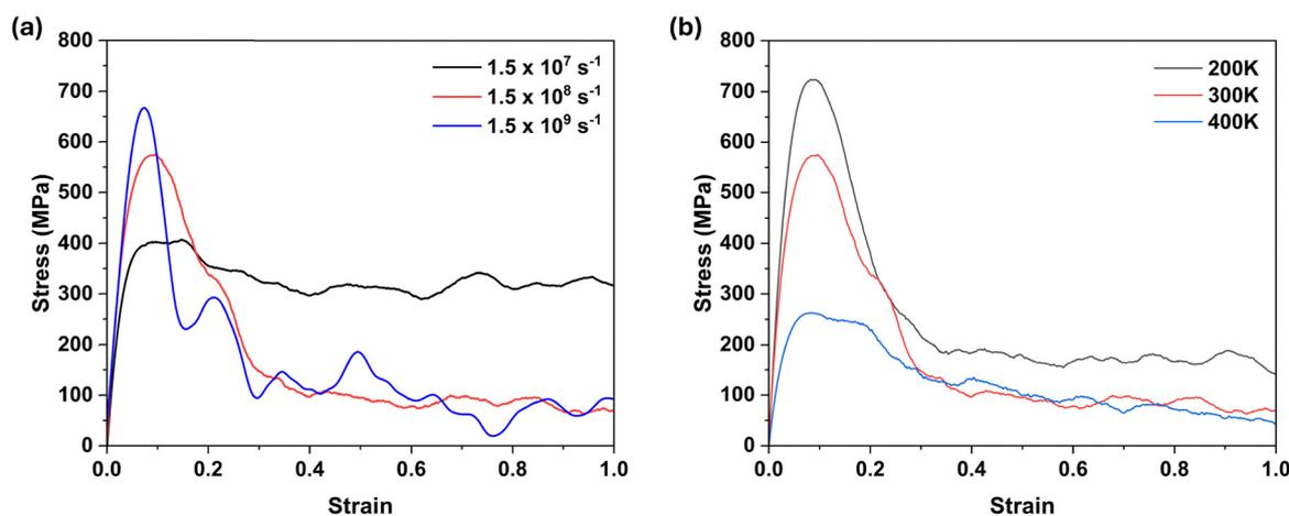
Fig. 5 Illustration of computed stress–strain curves for the 10% graphene-filled PVA nanocomposite (a) obtained by uniaxial tension at 300 K with three different strain rates viz.  $1.5 \times 10^7 \text{ s}^{-1}$ ,  $1.5 \times 10^8 \text{ s}^{-1}$ , and  $1.5 \times 10^9 \text{ s}^{-1}$  along the Cartesian X-axis; and (b) produced by uniaxial deformation at a strain rate of  $1.5 \times 10^8 \text{ s}^{-1}$  and the alteration of temperature.
