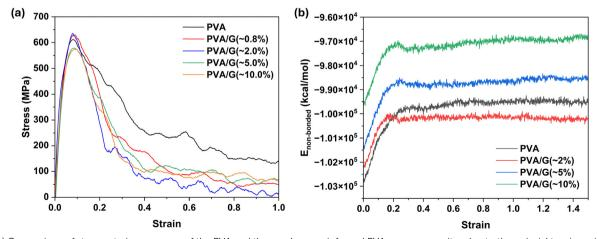
Fig. 3 (a) Comparison of stress-strain responses of the PVA and the graphene-reinforced PVA nanocomposites due to the uniaxial tension with a strain rate of  $1.5 \times 10^8$  s<sup>-1</sup> along the Cartesian X-axis of the simulation cell. (b) Illustration of changes in non-bonded energy ( $E_{non-bonded}$ ) as a function of strain for the PVA and the G-PVA nanocomposite comprising 2-10% graphene nanofiller.
