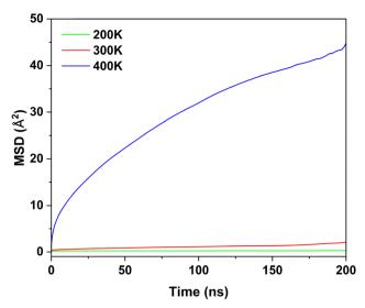
Fig. 6 Demonstration of temperature dependence of the calculated square displacement (MSD) curves for the PVA chains in the graphene-PVA composites comprising 10% graphene nanofiller.
