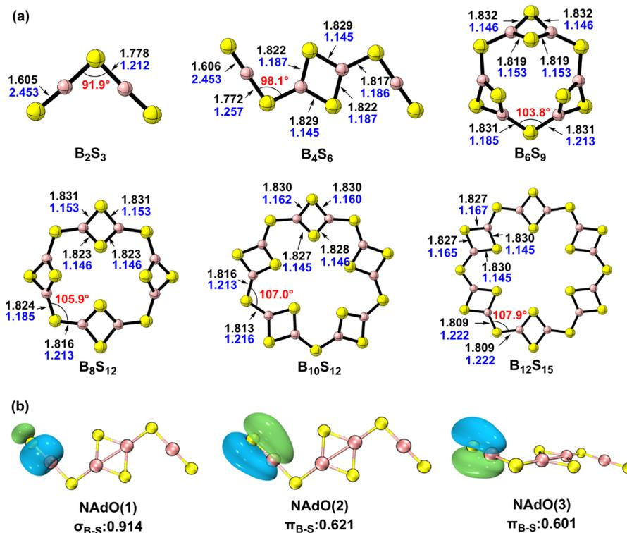
Fig. 2 (a) The optimized global minimum configurations of the studied  $(B_2S_3)_n$  clusters, where the key bond lengths (Å), Mayer bond orders, and bond angles ( $^\circ$ ) are given in black, blue, and red, respectively. (b) The NAdO analysis on the bonding modes of  $B_4S_6$  is given, where B and S atoms are in pink and yellow, respectively.
