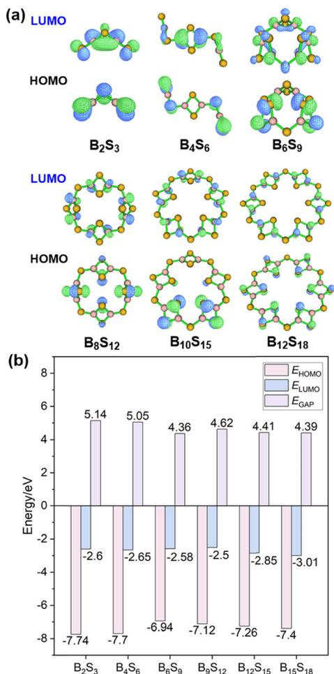
Fig. 4 (a) The key molecular orbitals (isosurface = 0.05) and (b) the corresponding energy levels (in eV) of the studied (B<sub>2</sub>S<sub>3</sub>)<sub>n</sub> clusters.
