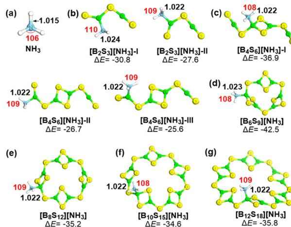
Fig. 6 The optimized structures and the relative energies ( $\Delta E$ , in  $\text{kcal mol}^{-1}$ ) of the  $NH_3$  molecule (a) and studied complexes  $[B_2S_3]_n[NH_3]$  (b–g), taking the energy sum of individual components as the reference. Key N–H bond lengths ( $\text{\AA}$ ) and H–N–H angles ( $^\circ$ ) are given in black and red, respectively. The color of atoms: S–yellow; B–green; N–blue; H–white.
