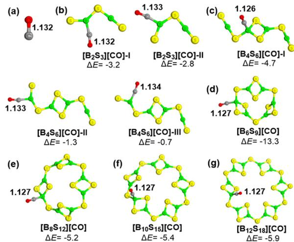
Fig. 7 The optimized structures of the CO molecule (a) and studied complexes  $[\text{B}_2\text{S}_3]_n[\text{CO}]$  (b–g), and their corresponding CO binding energies ( $\Delta E$ , in  $\text{kcal mol}^{-1}$ ), where key C–O bond lengths ( $\text{\AA}$ ) are given in black. The color of atoms: S–yellow; B–green; O–red.
