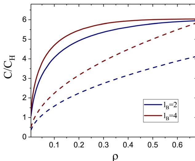
Fig. 4 The capacitance  $C/C_H$  obtained from (17) and (22) (solid lines) and  $C_D/C_H$  (dashed lines) as a function of the dimensionless density of ions for the Bjerrum length  $l_B = 2$  and  $l_B = 4$  in  $a$ -units.
