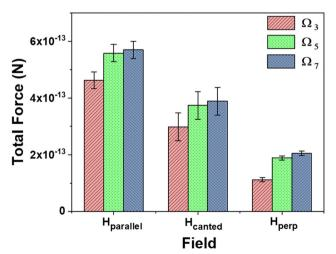
Fig. 8 Total forces for the various particle sizes ( $\Omega_{3}$ ,  $\Omega_{5}$ , and  $\Omega_{7}$ ) in dependence on the direction of the magnetic field acting on the sessile droplet during evaporation.
