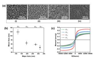
Fig. 2 (a) FE-SEM images of hematite nanoparticles of different shapes. (b) Dimensional measurement of anisotropic-shaped particles with aspect Major-axis length (2b) ratios of 1, 3, 5, and 7 denoted by  $\Omega_1$ ,  $\Omega_3$ ,  $\Omega_5$  and Minor-axis length (2a)  $\Omega_{7}$ , respectively. (c) The magnetization curve illustrates the magnetic behavior
