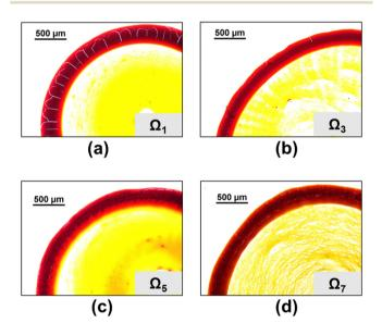
Fig. 3 Desiccation patterns of dried droplets containing anisotropicallyshaped nanoparticles with varying aspect ratios: (a)  $\Omega_1$ , (b)  $\Omega_3$ , (c)  $\Omega_5$ , and (d)  $\Omega_7$  in the absence of an external magnetic field. Fig. S1 in the ESI† shows magnified images for better visualization.
