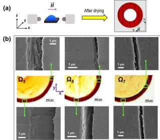
Fig. 5 (a) Schematic displaying the experimental setup with the magnet oriented parallel to the sessile droplet along the x-axis and the creation of the resulting deposition patterns. (b) FE-SEM and optical images illustrate the particle alignment and fracture direction during the deposition of various aspect ratios of 3, 5, and 7, respectively. For better observation of the deposition pattern, refer to Fig. S2-S4 in the ESI.†
