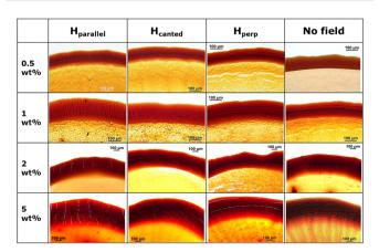
Fig. 9 Optical images illustrating crack propagation at the rim on the top side of the deposit as a function of varying concentrations of  $\Omega_7$  ferro-colloid suspension in the absence and presence of an external magnetic field
