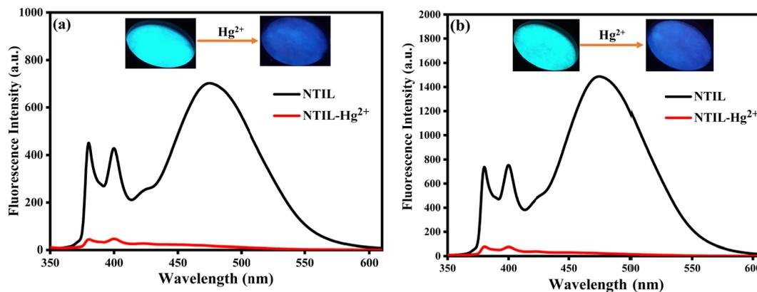
Fig. 9 (a) Fluorescent intensity and color variations of the paper strip with and without Hg<sup>2+</sup> ions (10<sup>-2</sup> M) in municipal water. (b) Fluorescent intensity and color variations of the paper strip with and without Hg<sup>2+</sup> ions (10<sup>-2</sup> M) in tap water.
