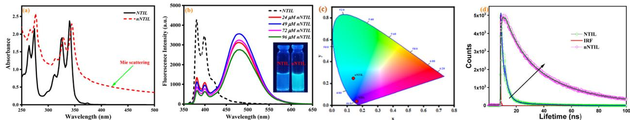
Fig. 1 (a) UV-visible absorption spectra of NTIL (49  $\mu\text{M}$ ) and nNTIL (49  $\mu\text{M}$ ). (b) Fluorescence spectra of NTIL and nNTIL in different amounts of NTIL. (c) CIE diagram of NTIL and nNTIL. (d) Photoluminescence lifetime decays of NTIL in THF and nNTIL in water.
