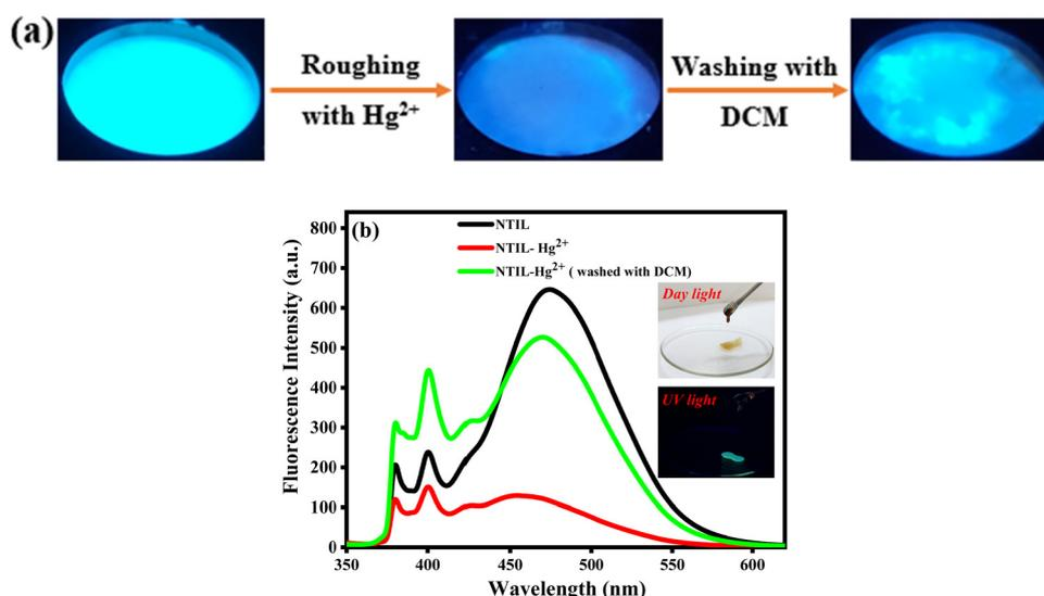
Fig. 10 (a) Photoluminescence characteristics of neat NTIL-loaded filter paper after roughening with Hg<sup>2+</sup> ions and its restoration following DCM washing. (b) Changes in the fluorescence intensity of the pure NTIL-loaded filter paper following treatment with mercury and its restoration after being washed with DCM. Inset: Images of neat NTIL in daylight and under UV light.
