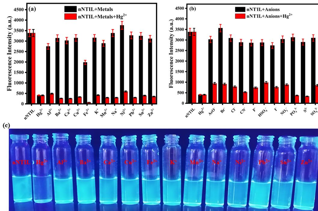
Fig. 6 Analysis of the interaction of nNTIL (49 μM) with Hg<sup>2+</sup> (113 μM) alongside different (a) metal ions (113 μM) and (b) anions (113 μM).  $\lambda_{\text{exc}} = 330$  nm, and  $\lambda_{\text{emi}} = 340$  nm. (c) Photograph showing the selectivity of nNTIL (49 μM) towards various metal ions (113 μM).
