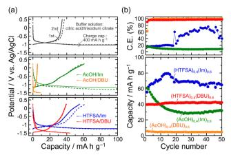
Fig. 4 (a) Galvanostatic charge/discharge (protonation/deprotonation) curves and (b) dependence of reversible capacities and coulombic efficiencies on cycle numbers for TiNb2O7 (hydrothermal) electrodes at a current density of 387 mA  $q^{-1}$  in the cut-off potential between -1.5 and +0.25 V vs. Ag/AgCl in sat. NaCl. For comparison, the electrochemical behavior in the aqueous buffer solution of 1 M citric acid and 1 M trisodium citrate is also shown
