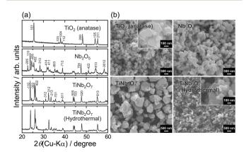
Fig. 2 (a) XRD patterns and (b) SEM images of TiNb<sub>2</sub>O<sub>7</sub> synthesized by different methods for comparison, the pattern and sem image of TiNb2O7 prepared by calcination is also shown
