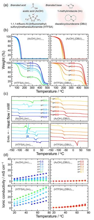
Fig. 1 (a) Chemical structures of Brønsted acid and base used in this study. (b) Thermogravimetric traces, (c) differential scanning calorimetry curves, and (d) ionic conductivities of  $(AcOH)_x(Im)_{1-x}$ ,  $(HTFSA)_x(Im)_{1-x}$  $(AcOH)_x(DBU)_{1-x}$ , and  $(HTFSA)_x(DBU)_{1-x}$  (x = 0.1, 0.2, 0.3, 0.4, 0.5).
