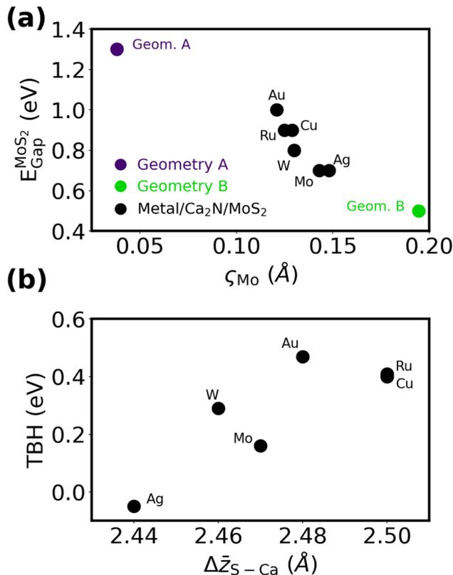
Fig. 6 (a)  $\text{MoS}_2$  band gaps in metal/ $\text{Ca}_2\text{N/MoS}_2$  heterostructures as a function of the honeycomb distortion; results for two  $\text{Ca}_2\text{N/MoS}_2$  heterobilayers are included for comparison. (b)  $\text{Ca}_2\text{N/MoS}_2$  tunneling barrier heights in metal/ $\text{Ca}_2\text{N/MoS}_2$  heterostructures as a function of the average vertical S–Ca separation.
