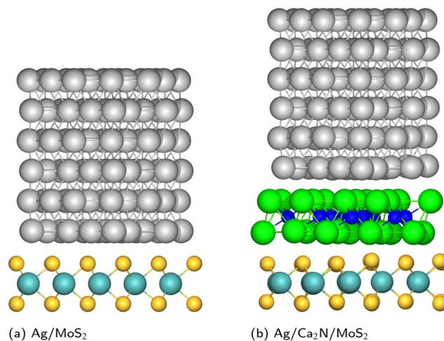
Fig. 1 Geometries of metal/MoS<sub>2</sub> and metal/Ca<sub>2</sub>N/MoS<sub>2</sub> heterostructures, for the specific case of Ag. Mo: cyan; S: yellow; Ag: silver; Ca: green; N: blue.
