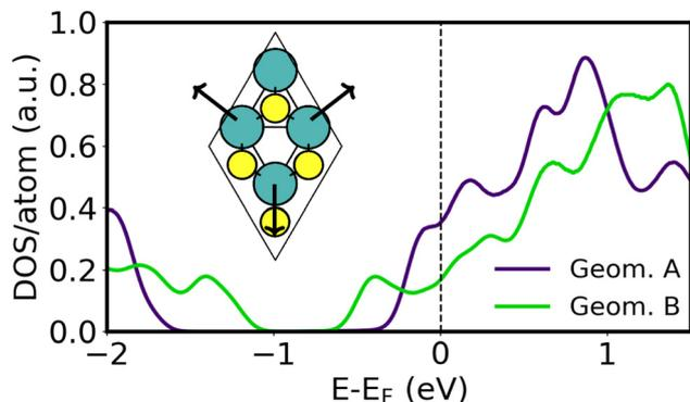
Fig. 3 MoS<sub>2</sub>-projected DOS for the two selected Ca<sub>2</sub>N/MoS<sub>2</sub> interface geometries. The computed DOS is divided by the total number of atoms in the heterobilayer due to the differing unit-cell sizes. The inset shows the honeycomb distortion present in Geometry B.
