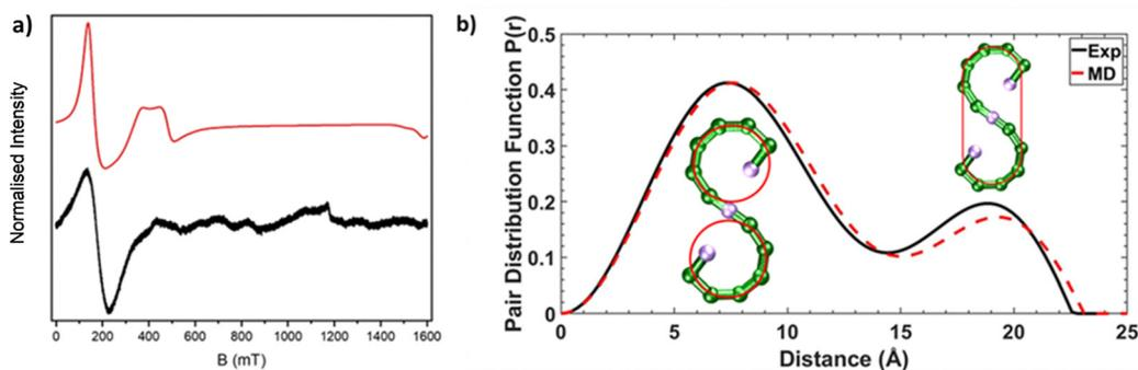
Fig. 2 (a) CW Q-Band (ca. 34 GHz) EPR spectra for **1** as a powder sample at 5 K, black line (experimental) and red line (simulation). (b) SAXS data for **1** presented as pair distribution functions (PDFs), measured (solid black line) and calculated from AMD simulations (dashed red line). The inserted schematics with red lines show atoms involved for the pair-pair distributions, at the corresponding distances in the PDFs.
