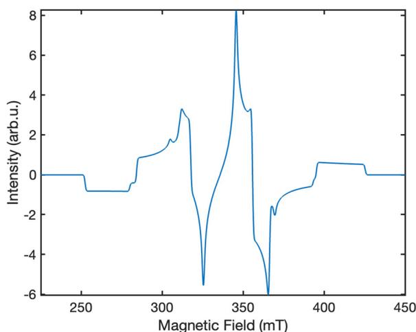
Fig. 6 The simulated powder-average EPR spectrum at ca. 300 ns for singlet fission in lycopene dimers using the “pepper” function in EasySpin.<sup>29</sup> The polarisation pattern predicted is EAEAEA. The intensity scale is presented in arbitrary units. The spectrometer frequency used in our simulation is  $\nu = 9.5$  GHz.
