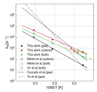
**Fig. 6** Arrhenius plot of the backbiting rate constants in a vacuum and the various solvents, namely o-/m-/p-xylene, BA monomer, and water at T = 310, 410, and 510 K. The results from this work are compared with experiments<sup>2,6,8</sup> and the theoretical predictions from ref. 12 and 13, which were obtained neglecting the presence of the solvent.
