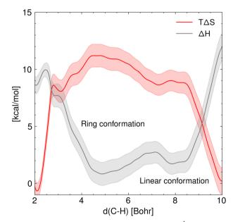
Fig. 5 Marginal entropy and enthalpy profiles [kcal  $mol^{-1}$ ] projected over the  $C_5$ -H distance in vacuum along with their standard deviation at  $T=410~\rm K$ . This plot highlights the opposing trends of enthalpy and entropy involved in the hydrogen transfer reaction.
