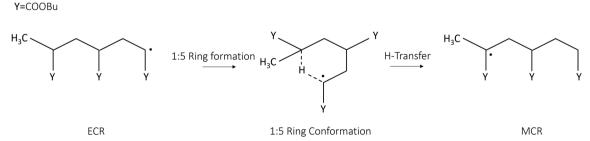
Fig. 2 Schematic representation of the 1:5 intramolecular hydrogen transfer (backbiting) of the BA model trimer, which is the model system used to study the reactivity of the poly-butyl acrylate. This chemical reaction requires the formation of a stable ring structure, enabling the hydrogen abstraction between the ECR and the MCR carbons
