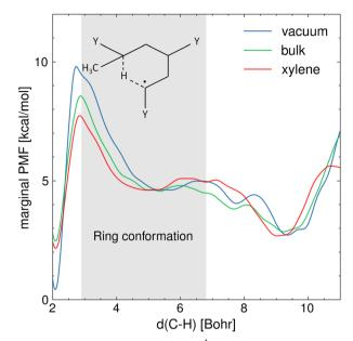
Fig. 4 Marginal PMF profiles [kcal  $mol^{-1}$ ], projected over the distance between the carbon radical ( $C_5$ ) and the hydrogen attached to  $C_1$  that is being transferred, in vacuum, in bulk and in xylene T=410 K. The gray area indicates the interval of  $C_5$ –H distances at which the 1:5 ring conformation is found, which is the precursor state to the hydrogen transfer.
