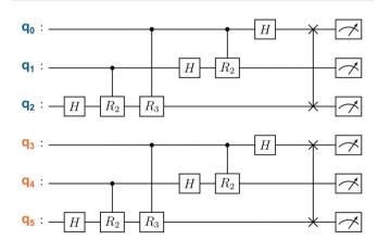
Fig. 2 Quantum circuit of 2-dimensional QFT for  $2^3 \times 2^3$  shaped input. Blue and orange letters correspond to bits along the x- and y-dimension. Vertical lines and boxes represent quantum operations.
