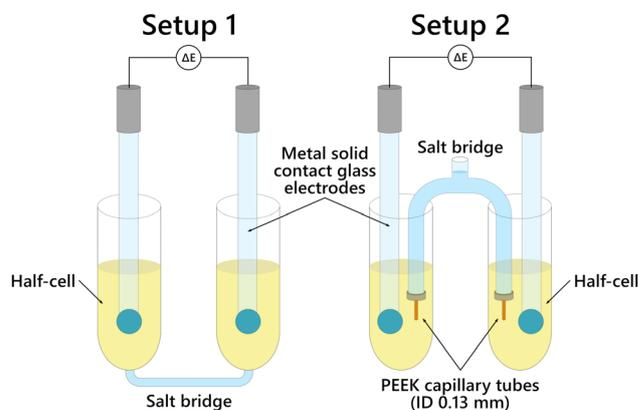
Fig. 1 Diagram of the salt bridge setups.
