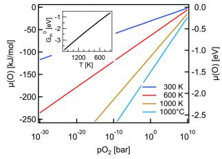
Fig. 1 Relationship between the oxygen chemical potential and the oxygen partial pressure as calculated from eqn (2) using data for the standard Gibbs energy of molecular oxygen<sup>22</sup> (100 kJ mol<sup>-1</sup> = 1.0364 eV  $\approx$  1 eV). The insert depicts the standard molar Gibbs energy of molecular oxygen,  $G_m^0(O_2) = \mu^0$ (data taken from ref. 22)
