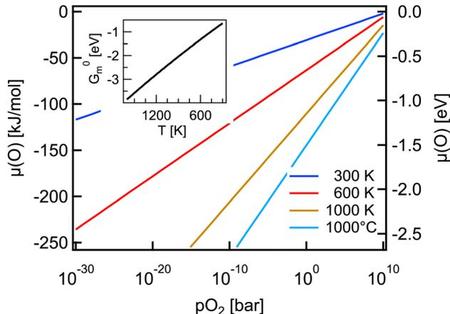
Fig. 1 Relationship between the oxygen chemical potential and the oxygen partial pressure as calculated from eqn (2) using data for the standard Gibbs energy of molecular oxygen<sup>22</sup> ( $100 \text{ kJ mol}^{-1} = 1.0364 \text{ eV} \approx 1 \text{ eV}$ ). The insert depicts the standard molar Gibbs energy of molecular oxygen,  $G_m^0(\text{O}_2) = \mu^0$  (data taken from ref. 22).
