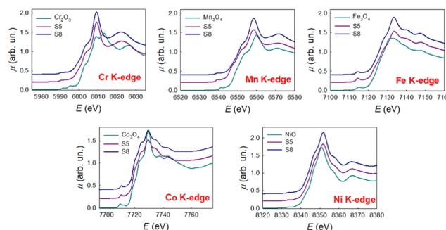
Fig. 1 Cr, Mn, Fe, Co and Ni K-edge XAS spectra of the S5 and S8 high entropy spinels at RT. The spectra of  $\text{Cr}_2\text{O}_3$ ,  $\text{Mn}_3\text{O}_4$ ,  $\text{Fe}_3\text{O}_4$ ,  $\text{Co}_3\text{O}_4$  and NiO are also shown for references of the oxidation state.
