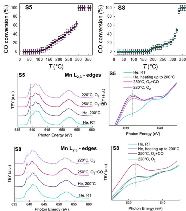
Fig. 4 CO oxidation activity and *operando* Mn  $L_{2,3}$ -edge XAS spectra of the S8 and S5 HEO materials: the energy region between 638.5 and 640.5 eV is shown on an enlarged energy scale for better evidencing the peak of Mn(II).
