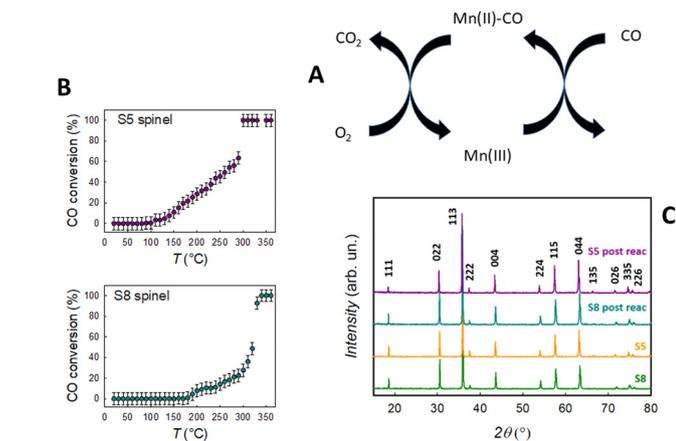
**Fig. 5** (A) Scheme of the catalytic cycle involving the Mn(II)/Mn(III) redox couple on the S5 and S8 high entropy spinels. (B) Comparison of the activity of the S5 and S8 spinels. The graph shows the time evolution of the ratio of the integrated area of the CG peaks of CO<sub>2</sub> and CO + O<sub>2</sub> over the two spinels. (C) X-ray powder diffraction patterns of the S5 and S8 spinels as prepared (yellow and green curves) and after (cyan and purple curves) the catalytic reaction.
