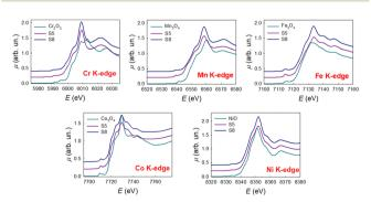
Fig. 1 Cr, Mn, Fe, Co and Ni K-edge XAS spectra of the S5 and S8 high entropy spinels at RT. The spectra of Cr<sub>2</sub>O<sub>3</sub>, Mn<sub>3</sub>O<sub>4</sub>, Fe<sub>3</sub>O<sub>4</sub>, Co<sub>3</sub>O<sub>4</sub> and NiO are also shown for references of the oxidation state
