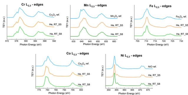
Fig. 2 Cr, Mn, Fe, Co and Ni  $L_{2,3}$ -edge XAS spectra of the S5 and S8 high entropy spinels at RT. The spectra of  $\text{Cr}_2\text{O}_3$ ,  $\text{Mn}_3\text{O}_4$ ,  $\text{Fe}_3\text{O}_4$ ,  $\text{Co}_3\text{O}_4$  and NiO are also shown for references of the oxidation state.
