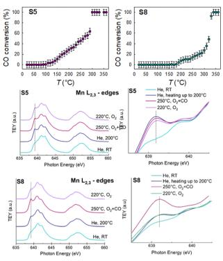
CO oxidation activity and operando Mn L<sub>2,3</sub>-edge XAS spectra of the S8 and S5 HEO materials: the energy region between 638.5 and 640.5 eV is shown on an enlarged energy scale for better evidencing the peak of Mn(II)
