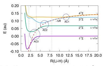
Fig. 2 FCI/aug-cc-pVTZ potential energy curves of the first four  $^1\Sigma$  states of LiH. The -1/R Coulombic tail, with zero at the Li^+-H^- reference energy, is also shown as a dashed line. The approximate position of the three avoided crossings is indicated with circles, and the distances at which a detailed analysis is provided in the text, are shown with dotted vertical lines.
