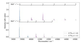
Fig. 6 Overview of the rovibrational energy-level structure of the BaH+ and BaD<sup>+</sup> X<sup>+</sup>  $^{1}\Sigma^{+}$  states obtained by PFI-ZEKE-PE spectroscopy following resonant two-photon excitation from the X  $^2\Sigma^+$  ground state of BaH/BaD via the E  ${}^{2}\Pi_{1/2}$  (v' = 0, 1) levels, as indicated by the colour code and the
