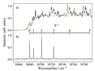
Fig. 5 Photoionisation (a) and PFI-ZEKE-photoelectron (b) spectra of  $^{138}$ BaH in the vicinity of the BaH $^+$  X $^+$   $^1\Sigma^+$  ( $v^+$  = 0) ionisation threshold and recorded from the BaH E  ${}^2\Pi_{1/2}$  (v'=0, N'=1, J'=1.5, –) intermediate level. The PFI-ZEKE-PE spectrum has been corrected for the field-induced shift of the ionisation thresholds. The wavenumber scale is with respect to the X  $^2\Sigma^+$  (v'' = 0, N'' = 0) ground state of BaH.
