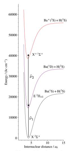
Fig. 1 Resonant multiphoton excitation scheme used to access the  $\text{X}^+\ ^1\!\Sigma^+$  ground state of  $\text{BaH}^+$  from the BaH X  $^2\Sigma^+$  ground state. The potential-energy curves are taken from ref. 18 and 44. An analogous excitation scheme was used in BaD to access the BaD<sup>+</sup> ground state.
