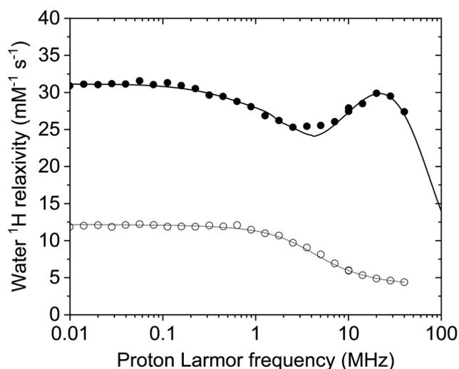
Fig. 7  $^1\text{H}$  relaxivity profiles of Gd-DOTA (empty symbols) and GdDOTA-conjugated ANSII (solid symbols) at  $25 \text{ }^\circ\text{C}$ . Best fit profiles obtained with the Florence NMRD program are also shown.<sup>21</sup>
