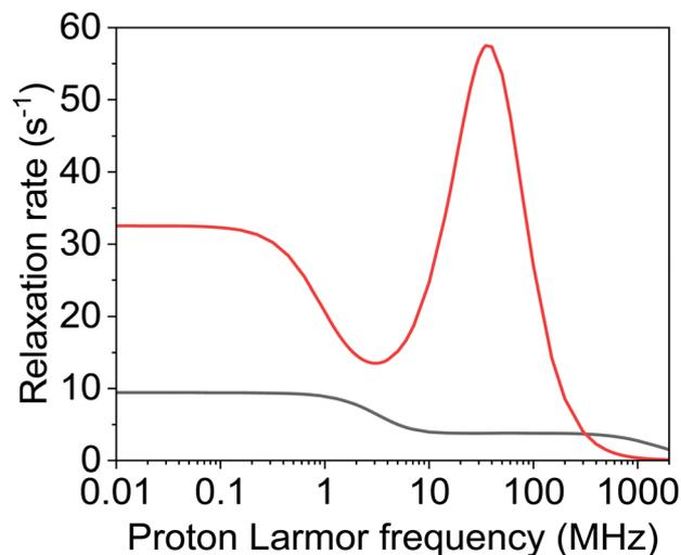
Fig. 5 Field dependence of the water proton relaxation rate ( $R_{1p}$ ) according to the SBM model (eqn (5)–(8)) for 1 water molecule coordinated to a  $Gd^{3+}$  ion ( $S = 7/2$ , in 1 mM concentration) at distance of 3.0 Å with  $\tau_M = 20$  ns,  $A_i = 0.02$  cm<sup>-1</sup>,  $\tau_v = 20$  ps and  $\tau_r$  of 100 ps (black line) or 3 ns (red line).
