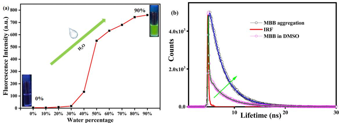
Fig. 5 (a) Emission intensity changes of probe **MBB** in the DMSO/H<sub>2</sub>O mixture with different percentages of water. Inset: Pictorial representation of the change of 0% water (colorless) and 90% water (green color) under UV light (365 nm). (b) Time-resolved fluorescence decay curve of the probe **MBB** and **MBB** aggregates at  $\lambda_{exc.} = 375$  nm.
