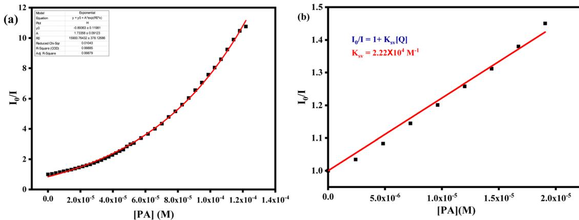
Fig. 11 (a) Stern–Volmer plot of the quenching of **MBB** microparticles on interaction with PA. (b) The linear Stern–Volmer curve of fluorescence quenching in the presence of a lower concentration of PA.
