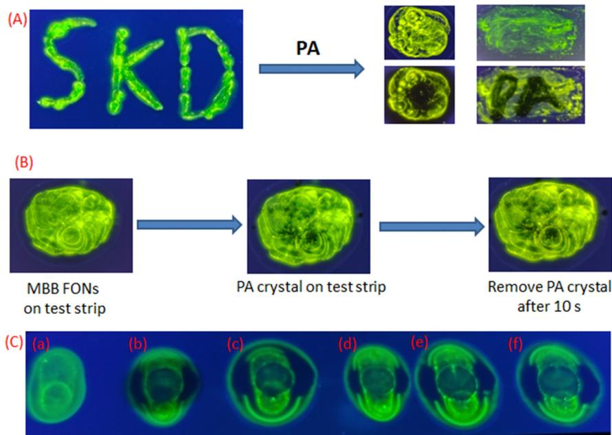
Fig. 14 (A) Pictorial representation of **MBB** water-suspended micromaterial absorbed test strip before and after the accumulation of PA. (B) Fluorescence image of the PA crystal on the test strip and after the removal of PA crystal after 10 s. (C) Fluorescence test strip image after introduction of various concentrations of PA: (a) **MBB** microparticles, (b)  $10^{-3}$ , (c)  $10^{-4}$ , (d)  $10^{-5}$ , (e)  $10^{-6}$ , and (f)  $10^{-7}$ .
