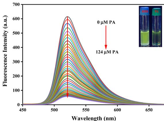
Fig. 9 Fluorescence titration spectra ( $\lambda_{\text{ex}} = 365$  nm) of fluorescent **MBB** microparticles (comprising 99% water) while introducing various concentrations of PA. Inset: Visualization of the change from robust green color fluorescence to non-fluorescence in the presence of PA.
