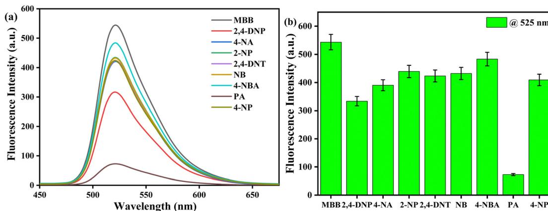
Fig. 10 (a) Emission spectra ( $\lambda_{\text{ex}} = 365$  nm) of **MBB** microparticles with several NACs. (b) Bar plot of fluorescence quenching of **MBB** microparticles after the addition of various NACs.
