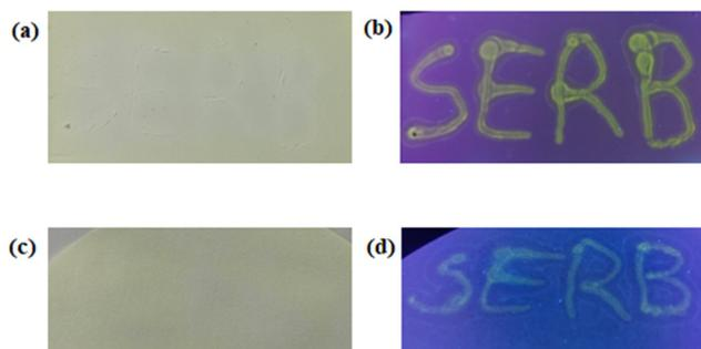
Fig. 2 Visibility of the word SERB, written using neat probe **MBB** in daylight (a) and (c) and under 365 nm UV light (b) and (d) on the surface of the TLC plate and Whatman-41 filter paper, respectively.
