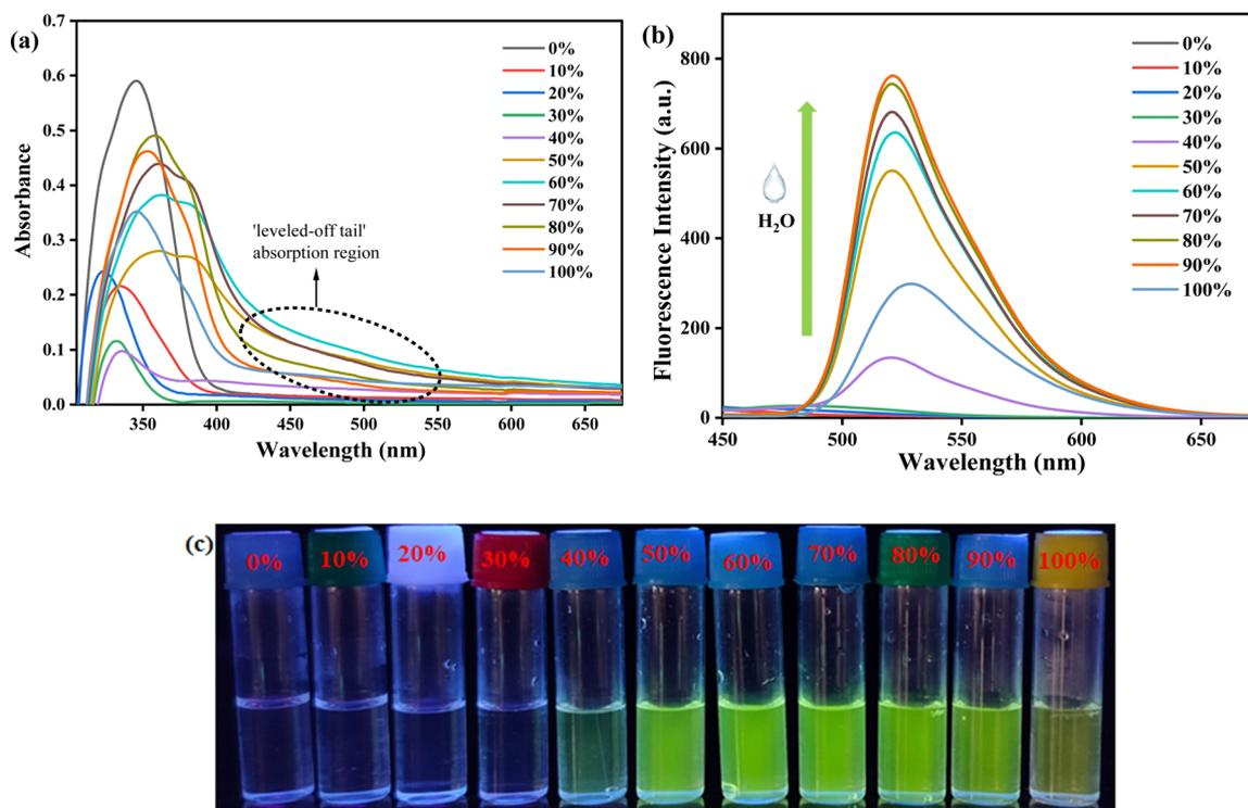
Fig. 4 (a) Changes in the absorbance spectrum of **MBB** upon increasing the water percentage in DMSO (from 0% to 100%). (b) Emission spectra of **MBB** in increasing aqueous medium (from 0% to 100%). (c) Pictorial representation of microparticle formation upon increasing the volume of water.
