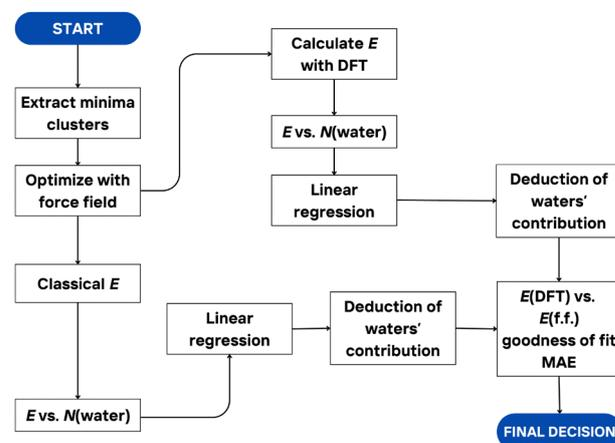
Fig. 1 Force field validation procedure (see text and ESI†).
