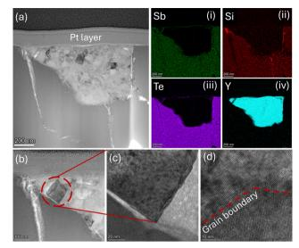
Fig. 2 (a) HRTEM image of Sb<sub>1.98</sub>Y<sub>0.02</sub>Si<sub>2</sub>Te<sub>6</sub>, and elemental mapping images showing the distribution of (i) Sb, (ii) Si, (iii) Te and (iv) Y. (b), (c) and (d) show the zoomed-in HRTEM images of the Y precipitate
