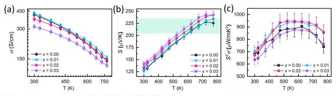
Fig. 3 Electronic transport properties of  $Sb_{2-x}Y_xSi_2Te_6$  (x = 0.00-0.03) with respect to temperature: (a) electrical conductivity, (b) Seebeck coefficient, and (c) power factor.
