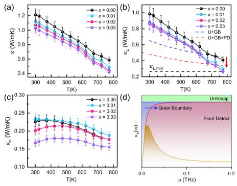
Fig. 5 (a) Thermal conductivity, (b) lattice thermal conductivity, (c) electronic thermal conductivity, and (d) Debye-Cahill modeling of lattice thermal conductivity of  $Sb_{2-x}Y_xSi_2Te_6$  (x = 0.0, 0.01, 0.02, and 0.03)
