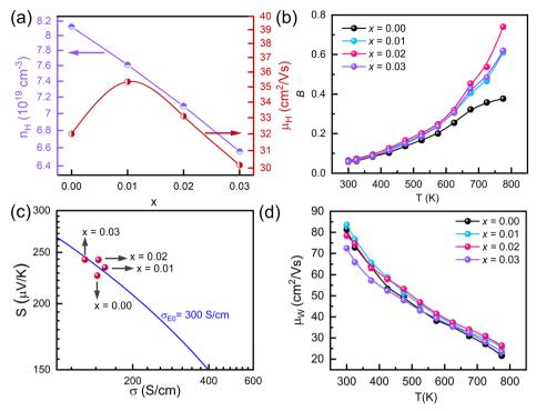
Fig. 4 (a) The carrier concentration and hall mobility with respect to carrier concentration, (b) quality factor values, (c) Jonker plot analysis, and (d) weighted mobility of  $Sb_{2-x}Y_xSi_2Te_6$  (x = 0.00, 0.01, 0.02, and 0.03).
