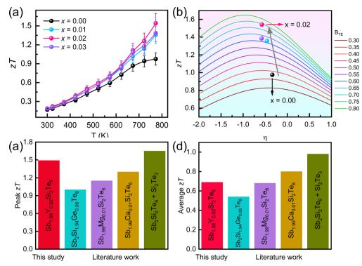
Fig. 6 (a) Thermoelectric figure of merit zT, (b) quality factor analysis showing the increase of zT values, (c) peak zT values, (d) average zT values of  $Sb_{2}Si_{2}Te_{6}\text{-related materials studied in the literature } (Sb_{1.98}Y_{0.02}Si_{2}Te_{6} \text{ (this study)}, \\ Sb_{2}Si_{1.94}Ge_{0.06}Te_{6}, \\ ^{39} \text{ and } Sb_{1.99}Mg_{0.01}Si_{2}Te_{6}, \\ ^{40} Sb_{1.99}Ca_{0.01}Si_{2}Te_{6}, \\ ^{5} Sb_{$
