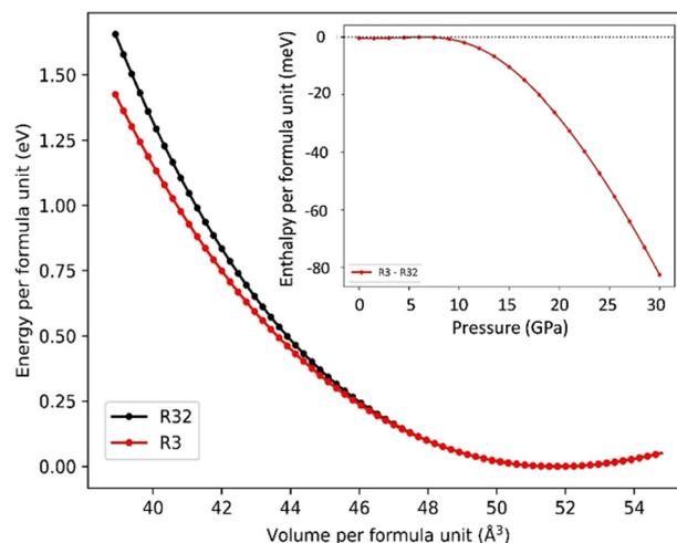
Fig. 10 DFT energy as a function of the volume per  $Mg_3Ca(CO_3)_4$  formula unit for the initial  $R32$  phase and the HP  $R3$  phase. Inset: Enthalpy difference as a function of pressure, showing the stability with respect to  $R32$   $Mg_3Ca(CO_3)_4$  huntite.
