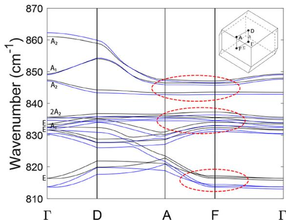
Fig. 11 Dispersion curves along a path in the Brillouin zone, including  $\Gamma(0\ 0\ 0)$ ,  $D(0\ 0\ 1/3)$ ,  $A(-1/2\ 1\ 1/3)$  and  $F(-1/2\ 1\ 0)$  points. Coordinates are given in fractional coordinates of the conventional (hexagonal) unit cell. Black and blue lines correspond to calculations at 7.6 and 11.1 GPa, respectively. Dashed red lines highlight states with a high density of states which may contribute to Raman dispersion.
