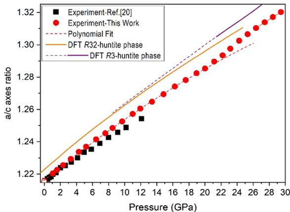
Fig. 5 Evolution of the  $a/c$  ratio of  $\text{Mg}_3\text{Ca}(\text{CO}_3)_4$  huntite with pressure. Black squares and red circles represent experimental data from a previous study<sup>20</sup> and the present study, respectively. The dashed line is a 2nd-order polynomial fitting to the low-pressure phase. The evolution of the DFT calculated ratios of both the initial  $R32$  and the predicted  $R3$  phases as a function of pressure are represented as orange and purple lines, respectively.
