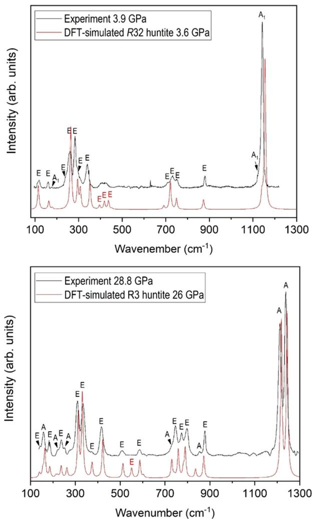
Fig. 9 Comparisons between calculated (red lines) and experimental (black lines) Raman spectra of the low-pressure  $R32$  (top) and the high-pressure  $R3$  (bottom) phases of  $Mg_3Ca(CO_3)_4$  at 3.9 and 28.8 GPa. Calculated Raman spectra were used for the mode assignment of Raman frequencies in the experiment.
