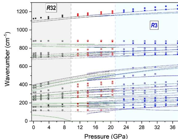
Fig. 8 Experimental (symbols) and calculated (lines) pressure dependence of the Raman-active modes of  $\text{Mg}_3\text{Ca}(\text{CO}_3)_4$ . Black and blue symbols represent bands of the initial *R32* huntite and the high-pressure *R3* phase, respectively. Red symbols correspond to the pressure range where most of the bands can be assigned to the initial *R32* huntite phase but small peaks and a band splitting in the  $[\text{CO}_3]$  bending frequency region appear.
