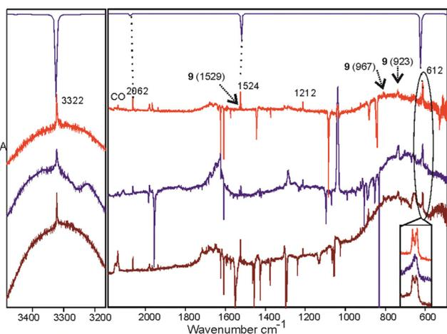
Fig. 10 Difference spectra depicting the identification of HC<sub>3</sub>P (7) among the products generated by far-UV photolyses (160–190 nm, 6-hour irradiations) of Ar-matrix isolated compounds 1 (bottommost, brown trace), 3 (red), and 5 (blue). Top: B3LYP/aug-cc-pVTZ prediction for the IR spectrum of 7 (frequency scaled by 0.96).
