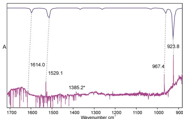
Fig. 11 Bottom: Difference spectrum (after-minus-before photolysis) showing, for phosphabutyne 1 in solid Ar, the net effect of an additional 24 h irradiation at 308 nm after 6 days of 254 nm photolysis. Top: B3LYP/aug-cc-pVTZ prediction for the IR spectrum of 9 (frequency scaled by 0.96). Asterisk assignment is tentative.
