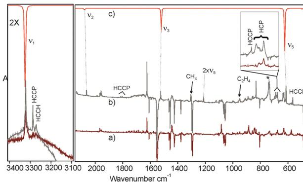
Fig. 9 Identification of the dissociation products observed upon UV photolysis of phosphabutryne (**1**) in solid argon. Traces (a) and (b) are different spectra (after-minus-before photolysis) illustrating the net effect of 3h and 76 h of Hg-lamp irradiation. Topmost trace shows the B3LYP/aug-cc-pVTZ prediction (frequency scaled by 0.96) for the IR spectrum of HC<sub>3</sub>P (**7**).
