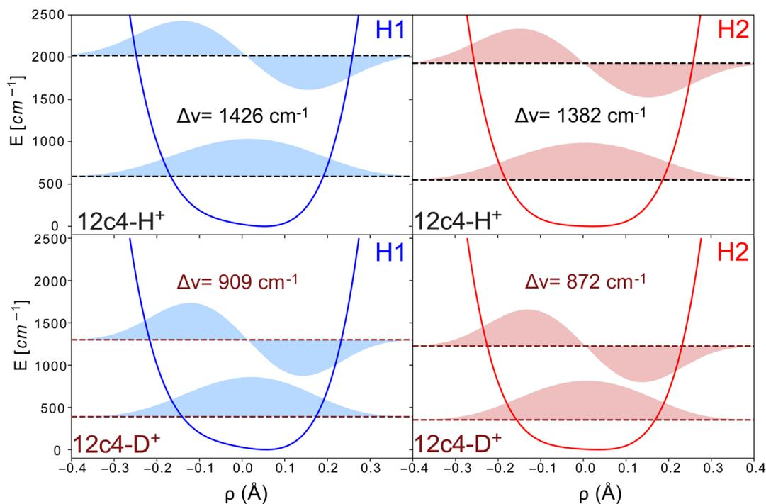
Fig. 6 Schematic representation of the potentials for the O- $H^+$ ...O stretching coordinate in the H1 and H2 structures, along with their corresponding eigenvectors and eigenvalues for the first two vibrational states, calculated using DVR computations (coordinate  $\rho$  defined as  $(R - r)/2$ ). The different panels depict the results for both conformers and H/D isotopologues.
