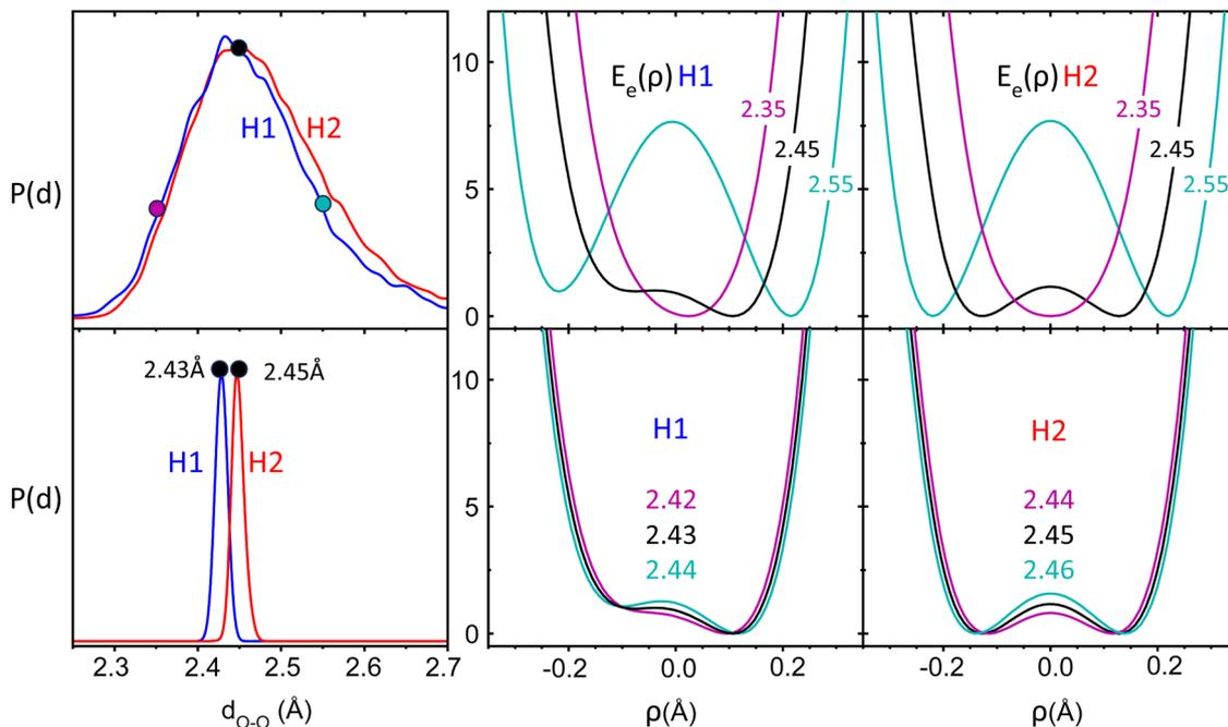
Fig. 5 Distribution of distances between the proton-bonded O atoms,  $P(d)$ , from BOMD computations of 12c4- $H^+$  in the H1 and H2 conformations at temperatures 350 K (top) and 1 K (bottom). Middle and right: Relaxed potential energy curves ( $\text{kJ mol}^{-1}$ ) for the proton in the intramolecular bond at fixed O-O distances representative of each temperature (coordinate  $\rho$  defined as  $(R - r)/2$ ).
