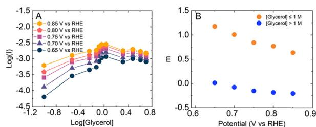
Fig. 5 (A) Dependence of log of current on log of glycerol concentration. (B) Potential dependence of reaction order ( $m$ ) for [Glycerol]  $\leq$  1 M (orange) and [Glycerol]  $>$  1 M (blue) concentrations (B).
