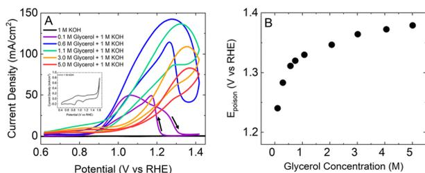
Fig. 4 (A) Cyclic voltammograms obtained from a polycrystalline Au disk in 1 M KOH +  $x$  M glycerol at a scan rate of 20 mV s<sup>-1</sup> with an inset blank voltammogram in 1 M KOH. (B) Potential of Au catalyst poisoning as a function of glycerol concentration.
