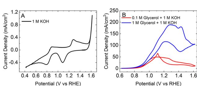
Fig. 6 Cyclic voltammogram obtained from a Au foil in a flow cell (2 mL min<sup>-1</sup>) at a scan rate of 50 mV s<sup>-1</sup> in (A) 1 M KOH and (B) 1 M KOH + 0.1 M glycerol (red) and 1 M KOH + 1 M glycerol (blue).
