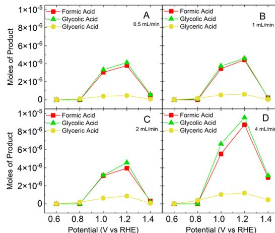
Fig. 11 Molar product distribution for glycerol electrooxidation on Au foil in a flow cell with 0.1 M glycerol + 1 M KOH at (A) 0.5 mL min<sup>-1</sup>, (B) 1 mL min<sup>-1</sup>, (C) 2 mL min<sup>-1</sup>, and (D) 4 mL min<sup>-1</sup> flow rates.
