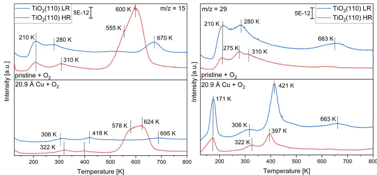
Fig. 5 TPR spectra of a monolayer methanol adsorbed at  $T = 115$  K and methanol with 56 L of oxygen pre-adsorbed at the pristine slightly (LR) and highly (HR) reduced  $\text{TiO}_2(110)$  single crystals (top spectra) and 20.9 Å of copper deposited onto the slightly and highly reduced single crystals (bottom spectra). Displayed are the  $m/z = 15$  and  $m/z = 29$  signals for the experiments reaching 800 K at a rate of  $2 \text{ K s}^{-1}$ .
