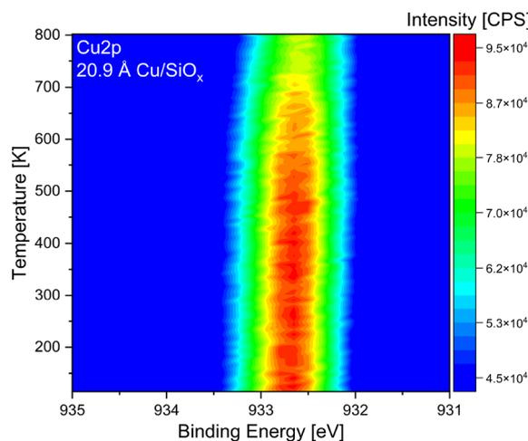
Fig. 1 Temperature-programmed X-ray photoelectron  $\text{Cu } 2p_{3/2}$  spectra after depositing 20.9 Å of copper onto a silicon wafer with a native oxide film. The sample was first cooled down to 120 K and then slowly heated to 800 K with a heating rate of  $0.5 \text{ K s}^{-1}$  while XP-spectra were recorded. All spectra loops were measured with a pass energy of 30, a step size of 0.15 eV and a dwell time of 25 ms.
