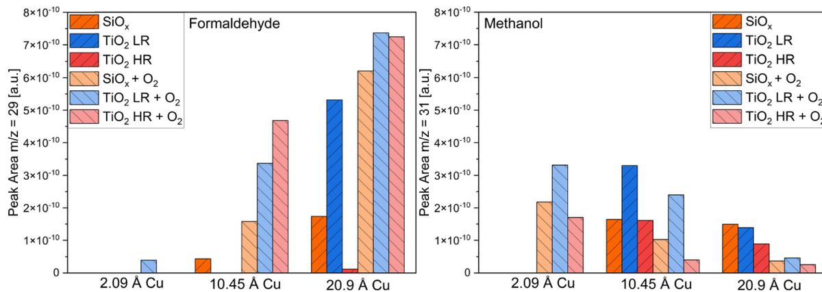
Fig. 6 Area of the observed peaks for the formaldehyde formation at  $m/z = 29$  and the methanol formation at  $m/z = 31$  when copper was deposited on the silicon wafer with a native oxide film (orange), on the slightly reduced  $\text{TiO}_2(110)$  (LR) single crystal (blue) and the highly reduced  $\text{TiO}_2(110)$  (HR) single crystal (red). The signal areas were taken from the spectra shown in this work and the ESI.†
