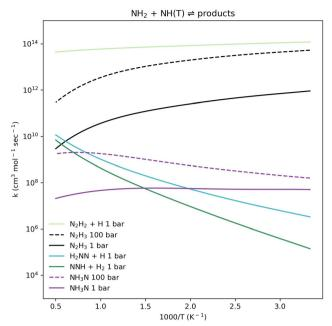
Fig. 6 Comparison of computed rate coefficients for unimolecular NH<sub>2</sub> + NH(T) reactions at 1 and 100 bar. Rate coefficients that do not exhibit a significant pressure-dependence in the examined range are only plotted at 1 bar. The  $N_2H_2 + H$  product channel shown here accounts for both trans and cis N2H2 isomers.
