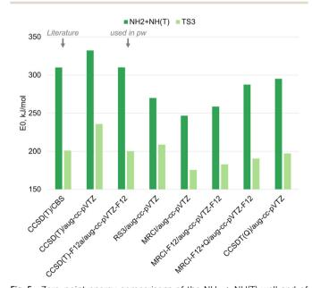
Fig. 5 Zero-point energy comparisons of the  $NH_2 + NH(T)$  well and of TS3, both relative to the zero-point energy of the  $N_2H_3$  isomer at the respective level. The CCSD(T)/CBS values were taken from Klippenstein et al. 52 (annotated as "Literature" in the figure). All other data were computed in the present work, and the CCSD(T)-F12a/aug-cc-pVTZ-F12 level of theory was further used for kinetic computations in the present work (annotated as "used in pw" in the figure).
