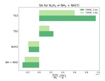
Fig. 10 Normalized sensitivity coefficients of the computed  $N_2H_3 \Rightarrow$ NH<sub>2</sub> + NH(T) rate coefficient evaluated with respect to the E0 values of all wells (the two isomers and bimolecular channels) as well as all TSs on the N<sub>2</sub>H<sub>3</sub> PES at 1000 and 1500 K, both at 1 bar. Only the highest normalized sensitivity coefficients are reported
