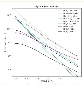
Fig. 7 Comparison of computed rate coefficients for unimolecular H<sub>2</sub>NN(S) + H reactions at 1 and 100 bar. Rate coefficients that do not exhibit a significant pressure-dependence in the examined range are only plotted at 1 bar. The N<sub>2</sub>H<sub>2</sub> + H product channel shown here accounts for both trans and cis N<sub>2</sub>H<sub>2</sub> isomers
