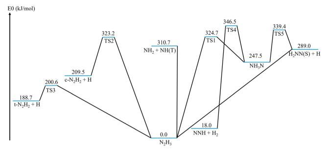
Fig. 2 The pressure-dependent kinetic network of the doublet N<sub>2</sub>H<sub>3</sub> PES computed at the CCSD(T)-F12a/aug-cc-pVTZ-F12//B2PLYP-D3/aug-cc-pVTZ level of theory. Zero-point energies (electronic energy plus zero-point energy correction) are in kJ mol<sup>-1</sup>.
