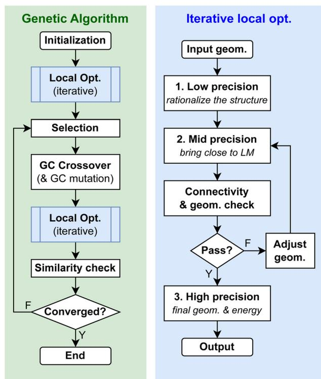
Fig. 7 The workflow of the GCGA evolution process and the iterative multi-stage local optimization process implemented in GOCIA.
