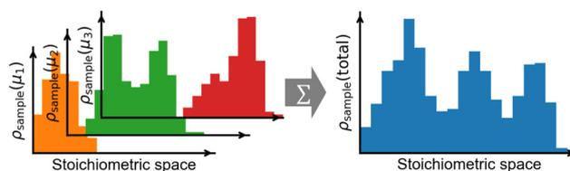
Fig. 6 The recommended practice for constructing a well-sampled GC ensemble. Multiple GC global optimizations are performed at a series of chemical potentials ( $\mu_n$ ,  $n = 1, 2, 3, \dots$ ). The samples (sub-ensembles) from multiple runs are then merged in to a total ensemble. If the sample distribution is continuous over the compositional space of interest, the merged ensemble can be used in the interpolated  $\mu$  range among  $\mu_n$ .
