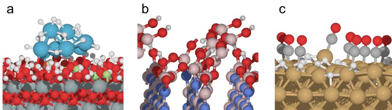
**Fig. 1** Examples of previous applications of GOCIA on catalytic systems. (a) H-covered Pt<sub>n</sub> clusters supported on hydroxylated F-doped tin oxide under electrochemical conditions. (b) Partially oxidized and hydroxylated over-layer of hexagonal boron nitride. (c) Restructuring of the crystalline Cu(100) surface under the coverage of a mixture of H and CO adsorbates.
