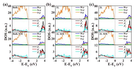
Fig. 2 (a)–(c) The LDOS and PDOS of bulk/1L/2L Bi<sub>2</sub>SeO<sub>5</sub>, respectively. The p orbitals of Bi, Se and O are projected in the LDOS and the  $p_x$ ,  $p_y$ , and  $p_z$ orbitals of Bi are projected in the PDOS. Note that the directions of  $p_x$ ,  $p_y$ , and  $p_z$  for the bulk system correspond to the b, c, and a directions (see Fig. 1a).
