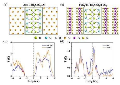
Fig. 3 (a) and (b) Schematic diagram and transmission spectra of the Al/1L Bi<sub>2</sub>SeO<sub>5</sub>/Al device. (c) and (d) Schematic diagram and transmission spectra of the FeS<sub>2</sub>/1L Bi<sub>2</sub>SeO<sub>5</sub>/FeS<sub>2</sub> MTJ.
