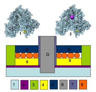
Fig. 12 The molecular vertical transistor (MolVeT) device. Top: Schematic of the un-doped (1) and C<sub>60</sub>-doped (2) bovine serum albumin (BSA). Bottom: C-Gate MolVet structure. The vertical transistor is formed inside a micro-cavity comprising highly doped silicon (1) covered with silicon dioxide (2) and surrounded by a silicon nitride layer (3). Au (4, Source), Pd (5, drain) and oxidized Ti (6,7, gate) electrodes are used to activate the protein layer (8) in the miniature junction
