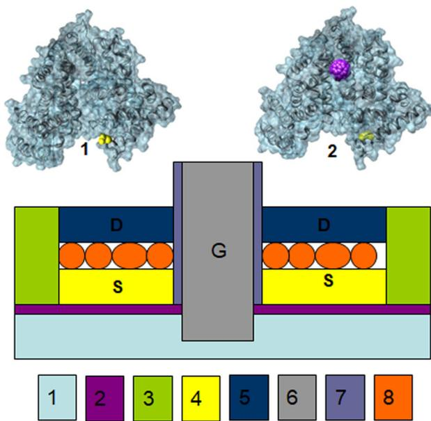
**Fig. 12** The molecular vertical transistor (MolVeT) device. Top: Schematic of the un-doped (1) and  $C_{60}$ -doped (2) bovine serum albumin (BSA). Bottom: C-Gate MolVeT structure. The vertical transistor is formed inside a micro-cavity comprising highly doped silicon (1) covered with silicon dioxide (2) and surrounded by a silicon nitride layer (3). Au (4, Source), Pd (5, drain) and oxidized Ti (6,7, gate) electrodes are used to activate the protein layer (8) in the miniature junction.
