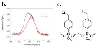
Fig. 5 Halogen desorption from molecular layers. (a) Halogen amount, normalized to the amount of Si, as a function of irradiation time, given on a log(t) scale for both I- and Cl-terminated SAMs. (b) The I 3d line recorded at different times of the experiment, I and II, demonstrating pronounced line-shape changes. (c) Molecules used for self-assembly on ITO. Taken from ref. 40.
