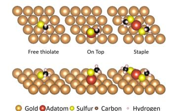
Fig. 2 The different forms in which the sulfur can attach to a Au(111) surface. Note that the binding sites for the thiolate vary between bridge site (free thiolate motif), hollow site (on-top motif) and on top of gold atoms (staple motif). The gold atoms are shown in brown, except for the gold adatom that is part of the thiolate motifs which is shown in red. The sulfur atoms are shown in yellow, the carbon atoms in black and the hydrogen atoms in pink.
