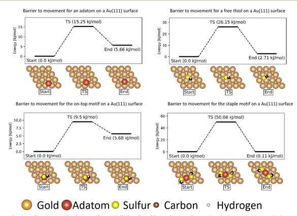
Fig. 3 Energy barriers of movement of various motifs on a Au(111) surface. All energies are referenced to the lowest energy state in the movement. The gold atoms are shown in brown, except for the gold adatom that is part of the thiol motifs which is shown in red. The sulfur atoms are shown in yellow, the carbon atoms in black and the hydrogen atoms in pink.
