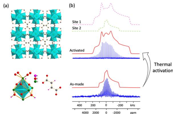
Fig. 5 (a) The long-range structure of MOF-801 (top) and local environments about Zr and the fumaric acid linker; (b) experimental (blue) and simulated (red) static <sup>91</sup>Zr NMR spectra of as-made and activated MOF-801 at 19.6 T, where an ECM was used to simulate the as-made MOF-801 spectrum.
