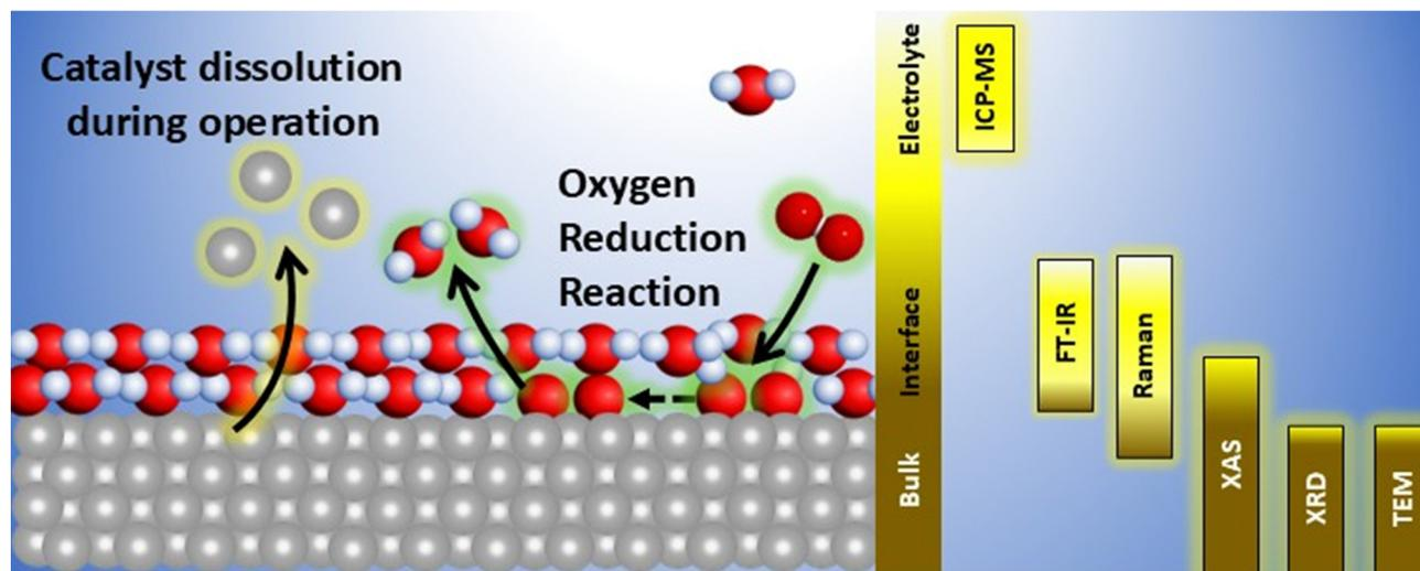
Fig. 2 Schematic representation of the electrode/electrolyte interface in electrocatalysis, and conventionally used *in situ/operando* techniques and the corresponding region probed. The oxygen reduction reaction (ORR) is sketched as example.
