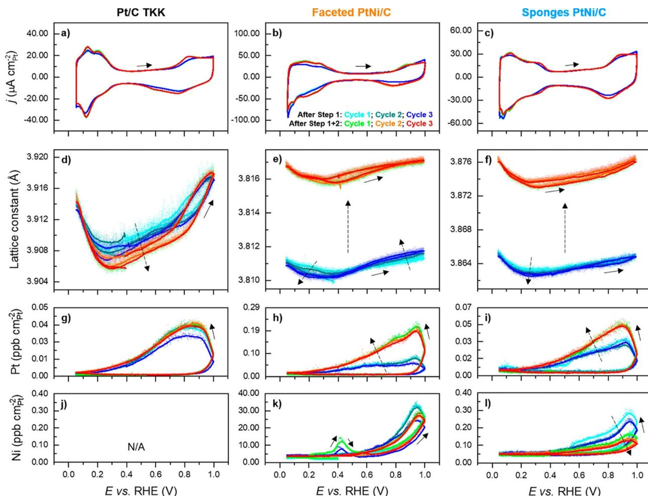
Fig. 4 (a)–(c) Cyclic voltammograms recorded at  $20 \text{ mV s}^{-1}$  using the RDE technique; (d)–(f) lattice strain dynamics measured using *operando* WAXS; specific dissolution profiles for (g)–(i) Pt and (j)–(l) Ni measured using online ICP–MS after protocol 1 (cyan, dark cyan, and blue traces) and protocol 1 + 2 (green, orange, and red traces) for Pt/C, faceted PtNi/C, and sponges PtNi/C catalysts. Reproduced with permission from ref. 23 Copyright 2022, American Chemistry Society.
