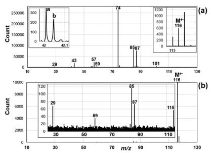
Fig. 2 Mass spectra of methyl valerate (Mr116) obtained by the (a) 15 eV EI and (b) SFTI method. The peaks labeled a and b in the insets represent fragment ions at m/z 42.0101 [C<sub>2</sub>H<sub>2</sub>O]<sup>+•</sup> and 42.0464 [C<sub>3</sub>H<sub>6</sub>]<sup>+•</sup>, respectively, which were separated by a high resolving power of 30 000 (FWHM) of the oTOF mass analyzer.
