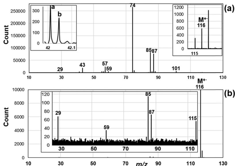
Fig. 2 Mass spectra of methyl valerate (Mr116) obtained by the (a) 15 eV EI and (b) SFTI method. The peaks labeled a and b in the insets represent fragment ions at  $m/z$  42.0101  $[C_2H_2O]^{\bullet+}$  and 42.0464  $[C_3H_6]^{\bullet+}$ , respectively, which were separated by a high resolving power of 30 000 (FWHM) of the oTOF mass analyzer.
