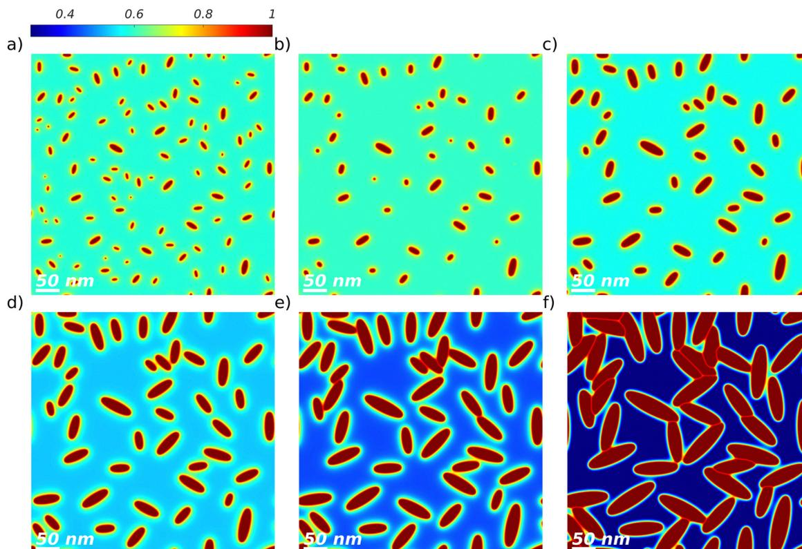
Fig. 2 TA at 140 °C of a binary DRCN5T : PC<sub>71</sub>BM blend with an initial blend ratio of 1 : 0.8, simulation of type A. The DRCN5T volume fraction fields are shown for the as-cast film with low crystal density (a) and after TA of 150 s (b), 300 s (c), 450 s (d), 600 s (e), and 900 s (f). The volume fraction colorbar spreads from dark blue (low DRCN5T content) to dark red (pure DRCN5T).
