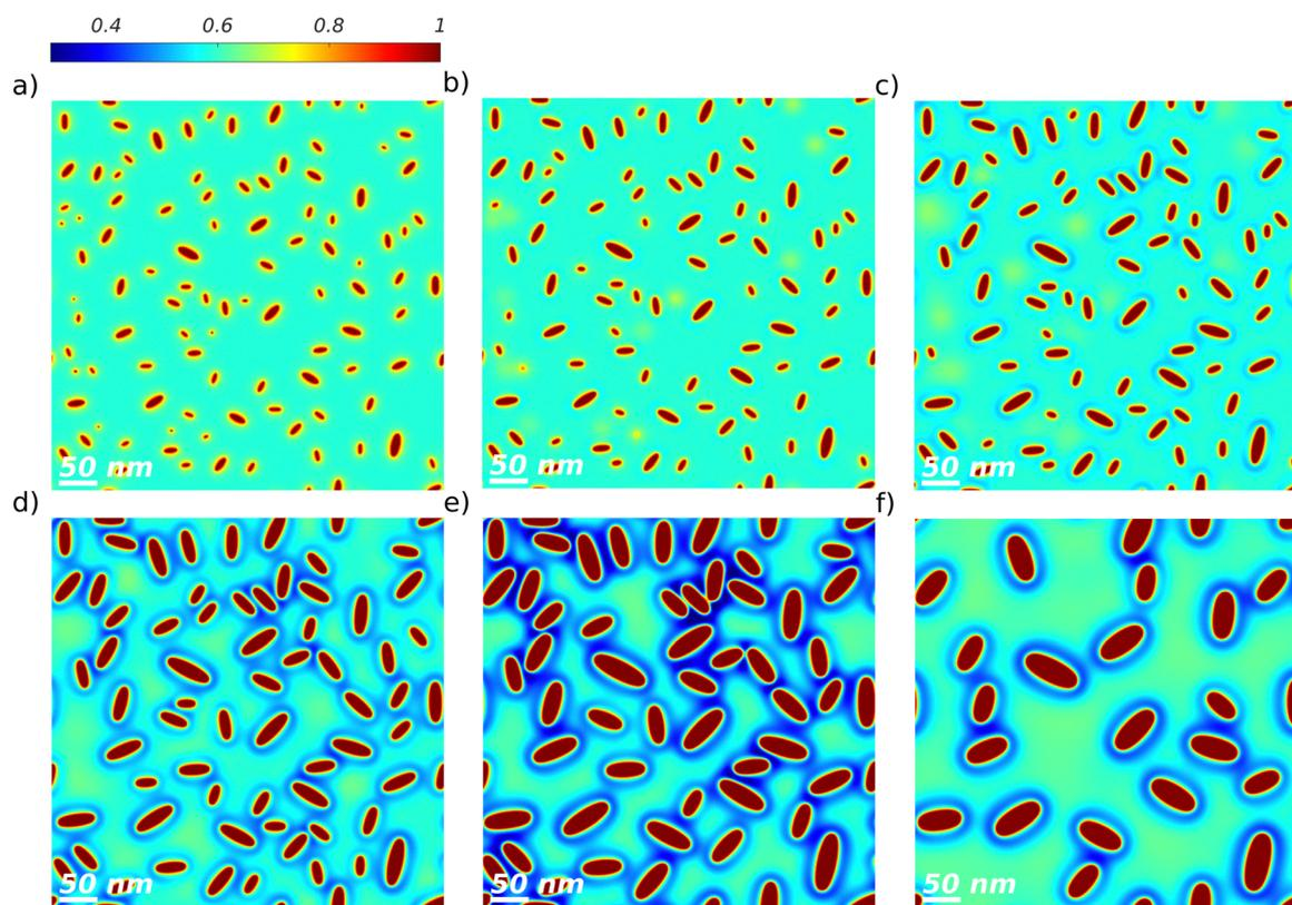
Fig. 9 TA of a binary DRCN5T : PC<sub>71</sub>BM blend with an initial blend ratio of 1 : 0.8, simulation of type E. The DRCN5T volume fraction fields are shown for the as-cast film with low crystal density (a) and after 600 s at TA temperatures of 80 °C (b), 100 °C (c), 120 °C (d), 140 °C (e), and 160 °C (f). The crystal growth is diffusion-limited. The volume fraction colorbar spreads from dark blue (low DRCN5T content) to dark red (pure DRCN5T).
