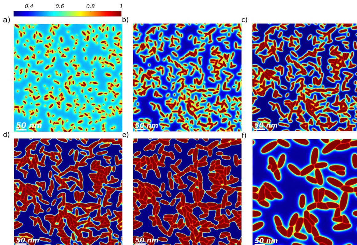
Fig. 6 TA of a binary DRCN5T : PC<sub>71</sub>BM blend with an initial blend ratio of 1 : 0.8, simulation of type B. The DRCN5T volume fraction fields are shown for the as-cast film with high crystal density (a) and after 600 s at TA temperatures of 80 °C (b), 100 °C (c), 120 °C (d), 140 °C (e), and 160 °C (f). The volume fraction colorbar spreads from dark blue (low DRCN5T content) to dark red (pure DRCN5T).
