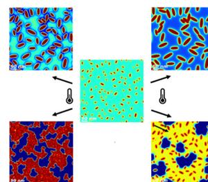
Fig. 1 Simulated DRCN5T:PC<sub>71</sub>BM morphologies under various thermal annealing conditions. The centered image corresponds to the as-cast simulated film, the other images correspond to the morphology after thermal annealing under diffusion limited (top left corner) and normal crystal growth (top right corner) regimes, with nucleation (bottom left corner) and with amorphous–amorphous phase separation (bottom right corner).
