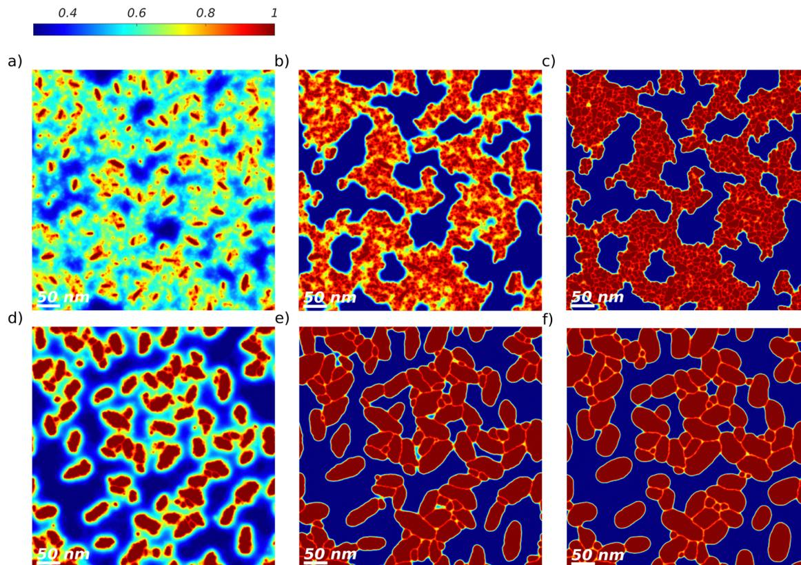
Fig. 7 TA at 80 °C (top row) and 140 °C (bottom row) of a binary DRCN5T:PC<sub>71</sub>BM blend with an initial blend ratio of 1:0.8, simulation of type C. The DRCN5T volume fraction fields are shown, after TA of 150 s (a) and (d), 300 s (b) and (e), and 600 s (c) and (f). The volume fraction colorbar spreads from dark blue (low DRCN5T content) to dark red (pure DRCN5T).
