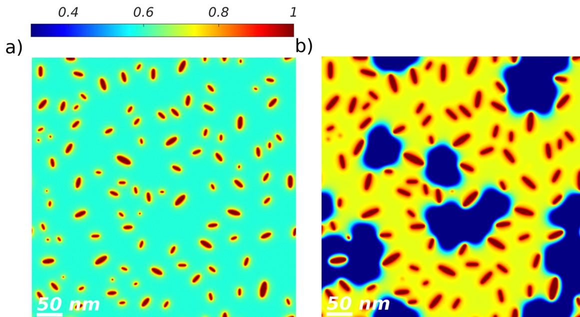
Fig. 8 TA at 80 °C of a binary DRCN5T : PC<sub>71</sub>BM blend with an initial blend ratio of 1 : 0.8, simulation of type D. The DRCN5T volume fraction fields are shown for the as-cast film with low crystals density (a) and at a TA time of 600 s (b). The volume fraction colorbar spreads from dark blue (low DRCN5T content) to dark red (pure DRCN5T).
