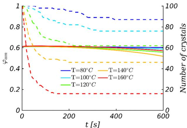
Fig. 4 Time-dependent DRCN5T volume fraction in the amorphous phase  $\varphi_{am}$  (solid line and left y-axis) and the number of DRCN5T crystals (dashed line and right y-axis) for different annealing temperatures.
